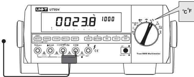
Figure 3-15. Temperature Measurement
