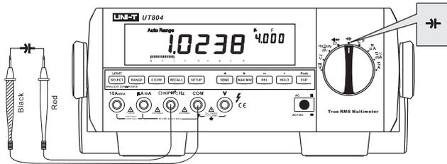
Figure 3-13. Capacitance Measurement
