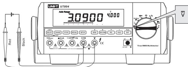
Figure 3-1. DC Voltage Measurement
