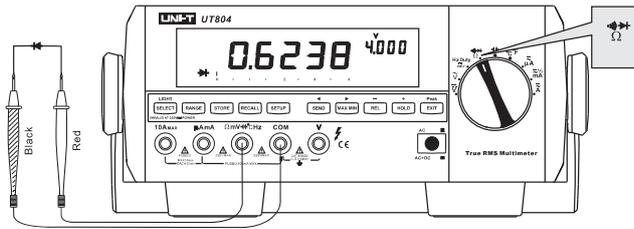
Figure 3-12. Diode Test
