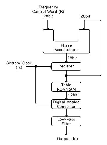
The phase accumulator adds the frequency control word K at every clock cycle fs. The accumulator output points to a location in the Table ROM/RAM. The DAC converts the digital data into an analog waveform. The LPF filters out the clock frequency to provide a pure waveform.
