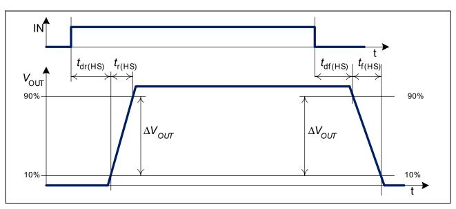
Figure 5 Definition of switching times high side (R<sub>load</sub> to GND)
