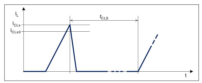
Figure 7 Timing Diagram Current Limitation
