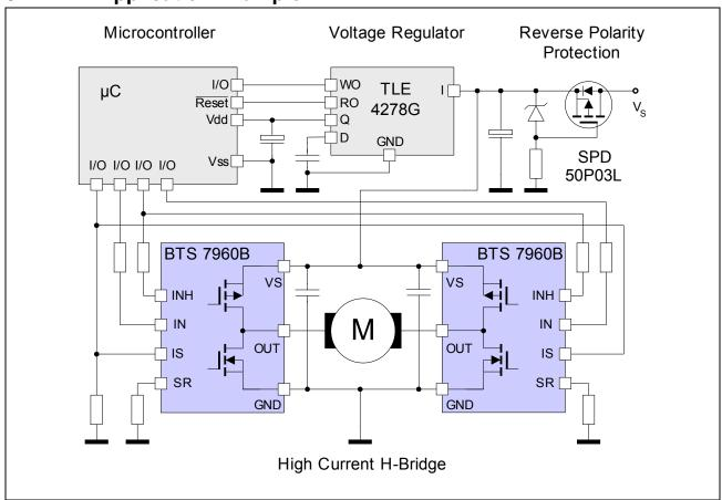
Figure 11 Application Example: H-Bridge with two BTS 7960B
