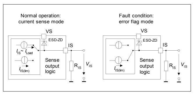
Figure 10 Sense current and fault current
