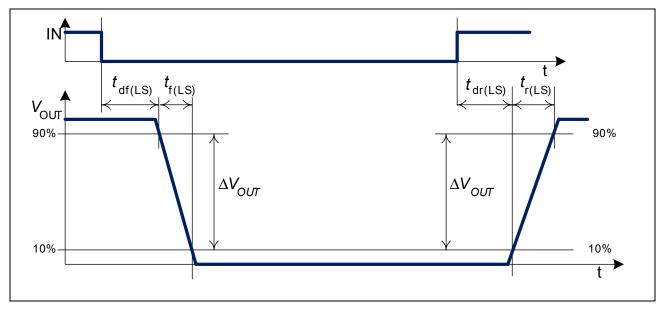
Figure 6 Definition of switching times low side (R<sub>load</sub> to VS)
