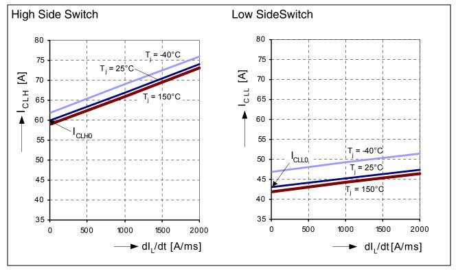
Figure 8 Current Limitation Level vs. Current Slew Rate dl/dt
