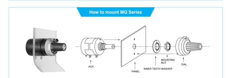
After the potentiometer is fixed to the panel using the mounting nut, the shaft of the potentiometer is turned anticlockwise to its limit and is put into the mounting hole of the dial which was already set at "0". The shaft of the potentiometer is secured by the screw positioned at the knob of the dial with the attached hexagonal wrench. With this, the mounting is completed.
