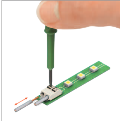
Inserting/removing fine-stranded conductors by lightly pressing on push-button (e.g., using a 233-335 operating tool or a ball point pen).
