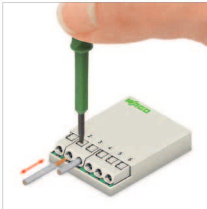
Inserting/removing fine-stranded conductors by lightly pressing on push-button (e.g., using a 233-335 operating tool or a ball point pen).
