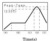
to the following (230 deg.C or more) graph. (E)Cooling zone 200 deg.C to 100 deg.C 1 deg.C/s to 4 deg.C/s
