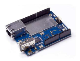
text based formats like XML that require quite a lot or ram to parse. On the Arduino YÚN we have created the Bridge library which delegates all network connections and processing of HTTP transactions to the Linux machine.
