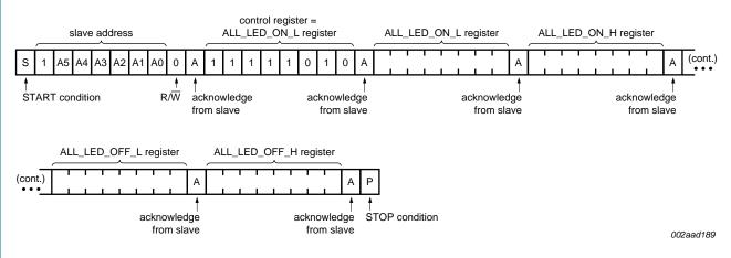
Fig 23. Write to ALL\_LED\_ON and ALL\_LED\_OFF registers using the Auto-Increment feature; AI initially set
