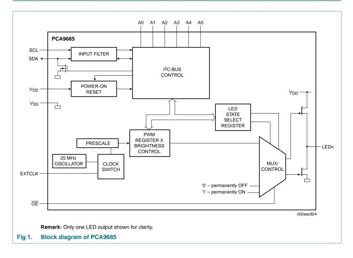
16-channel, 12-bit PWM Fm+ I<sup>2</sup>C-bus LED controller
