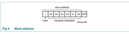
The last bit of the address byte defines the operation to be performed. When set to logic 1 a read is selected, while a logic 0 selects a write operation.
