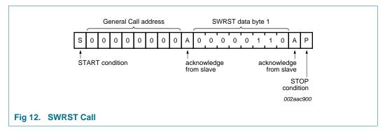
The I<sup>2</sup>C-bus master must interpret a non-acknowledge from the PCA9685 (at any time) as a 'SWRST Call Abort'. The PCA9685 does not initiate a reset of its registers. This happens only when the format of the SWRST Call sequence is not correct.
