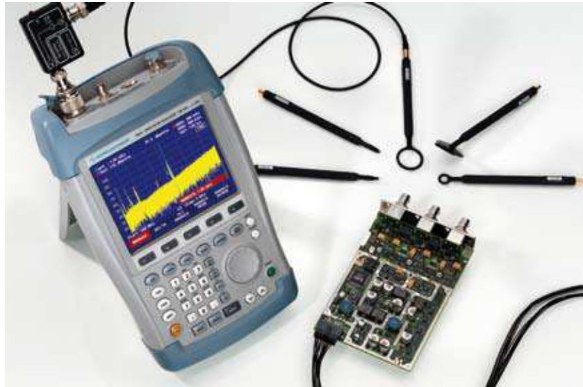
Near-field Probe Set R&S® HZ-15 with Spectrum Analyzer R&S® FSH3 and Preamplifier R&S® HZ-16
