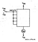
Fig. 29-Quiescent device current test circuit.
