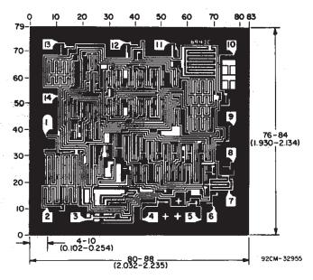
Chip dimensions and pad layout for CD4047B
