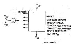
Fig. 31—Input-leakage-current test circuit
