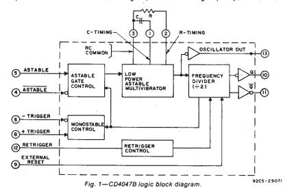
Fig. 2—CD4047B logic diagram.
