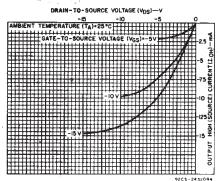
Fig. 6—Typical output high (source) current characteristics.
