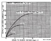
Fig. 4—Typical output low (sink) current characteristics.
