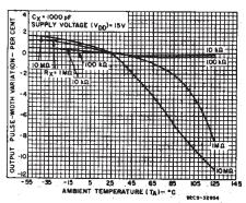
Fig. 25—Typical output pulse-width variations vs. ambient temperature.
