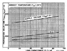
Fig. 9—Typical propagation delay time as a function of load capacitance (+ or - trigger to Q, \overline{Q}).
