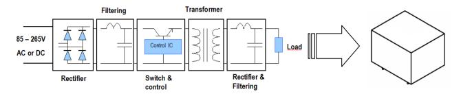
MYRRA encapsulated electronic transformers are Switched Mode Power Supplies based on Flyback topology.
