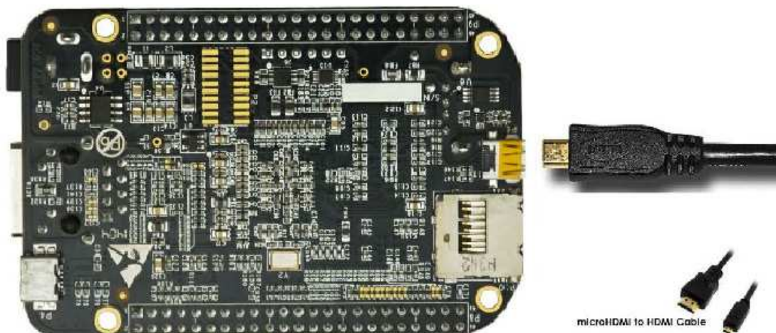
Figure 14 Connect microHDMI Cable to the Board
