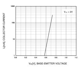
Figure 4. Base-Emitter On Voltage
