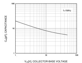
Figure 5. Collector Output Capacitance
