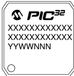
100-Lead TQFP (12x12x1 mm)
