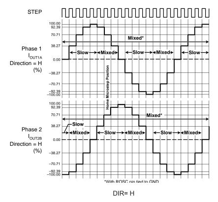
Figure 10. Decay Modes for Quarter-Step Increments
