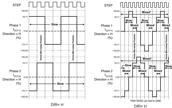
Figure 8. Decay Mode for Full-Step Increments
