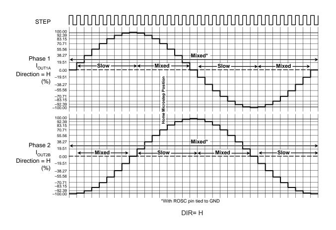
Figure 11. Decay Modes for Eighth-Step Increments
