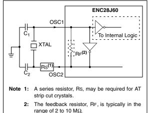
FIGURE 2-2: EXTERNAL CLOCK SOURCE<sup>(1)</sup>
