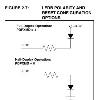
The LEDs can also be configured separately to control their operating polarity (on or off when active), blink rate and blink stretch interval. The options are controlled by the LACFG3:LACFG0 and LBCFG3:LBCFG0 bits. Typical values for blink stretch are listed in Table 2-1.
