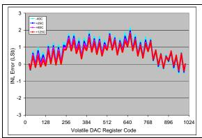
**FIGURE 2-20:** INL vs. Code (code = 25 to 1000) and Temperature (MCP4716).  $V_{DD} = 5V$ ,  $V_{REF1}$ :  $V_{REF0} = '10'$ , G = '0',  $V_{REF} = V_{DD}$ .
