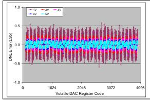
**FIGURE 2-70:** DNL vs. Code (code = 100 to 4000) and  $V_{REF}$  (**MCP4726**).  $V_{DD} = 5V$ ,  $V_{REF1}$ : $V_{REF0} = '10'$ , G = '0',  $V_{REF} = 1V$ , 2V, 3V, 4V, and 5V,  $T_{REF0} = +25$  °C.
