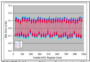
**FIGURE 2-29:** DNL vs. Code (code = 25 to 1000) and Temperature (MCP4716).  $V_{DD} = 2.7V$ ,  $V_{REF1}$ :  $V_{REF0} = '10'$ , G = '0',  $V_{REF} = V_{DD}$ .
