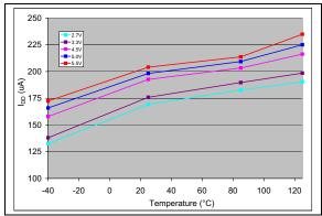
**FIGURE 2-88:**  $I_{DD}$  vs. Temperature.  $V_{DD} = 2.7V$  and 5V,  $V_{REF1}$ : $V_{REF0} = '00'$ .
