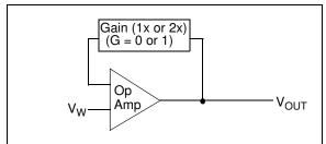
**FIGURE 4-4:** Output Buffer Block Diagram.
