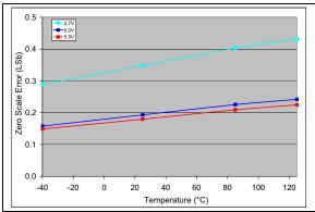
FIGURE 2-32: Zero Scale Error (ZSE) vs. Temperature (MCP4716).
