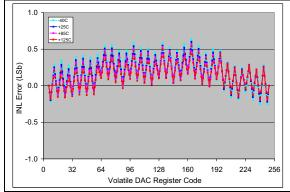
**FIGURE 2-24:** INL vs. Code (code = 6 to 250) and Temperature (MCP4706).  $V_{DD} = 2.7V$ ,  $V_{REF1}$ : $V_{REF0} = '10'$ , G = '0',  $V_{REF} = V_{DD}$ .
