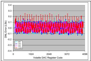
**FIGURE 2-43:** DNL vs. Code (code = 100 to 4000) and Temperature (**MCP4726**).  $V_{DD} = 5V$ ,  $V_{REF1}$ : $V_{REF0} = '11'$ , G = '0',  $V_{REF} = V_{DD}$ .
