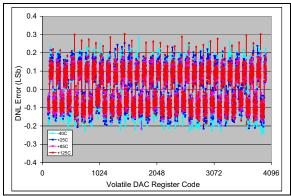
**FIGURE 2-28:** DNL vs. Code (code = 100 to 4000) and Temperature (**MCP4726**).  $V_{DD} = 2.7V$ ,  $V_{REF1}$ :  $V_{REF0} = '10'$ , G = '0',  $V_{REF} = V_{DD}$ .
