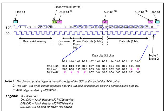
FIGURE 6-1: Write Volatile DAC Register Command.
