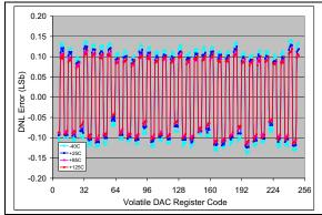
**FIGURE 2-12:** DNL vs. Code (code = 6 to 250) and Temperature (MCP4706).  $V_{DD} = 2.7V$ ,  $V_{REF1}$ :  $V_{REF0} = '00'$ .
