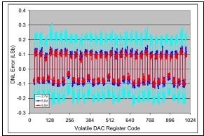
**FIGURE 2-65:** DNL vs. Code (code = 25 to 1000) and  $V_{DD}$  (2.7V, 5V, 5.5V) (MCP4716).  $V_{REF1}$ : $V_{REF0}$  = '11', G = '1',  $V_{REF}$  =  $V_{DD}$ /2,  $T_{CMD}$  = +25 °C.
