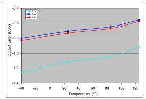
**FIGURE 2-81:** Output Error vs. Temperature (MCP4706).  $V_{DD} = 2.7V$  and 5V,  $V_{RFF1}$ :  $V_{RFF0} = '00'$ , Code = 250.
