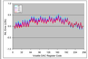
FIGURE 2-39: INL vs. Code (code = 6 to 250) and Temperature (MCP4706).  $V_{DD} = 5V$ ,  $V_{REF1}$ :  $V_{REF0} = '11'$ , G = '0',  $V_{REF} = V_{DD}$ .
