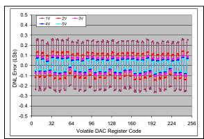
**FIGURE 2-72:** DNL vs. Code (code = 6 to 250) and  $V_{REF}$  (MCP4706).  $V_{DD} = 5V$ ,  $V_{REF1}$ : $V_{REF0} = '10'$ , G = '0',  $V_{REF} = 1V$ , 2V, 3V, 4V, and 5V,  $T_{EMD} = +25$  °C.
