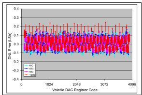
FIGURE 2-7: DNL vs. Code (code = 100 to 4000) and Temperature (MCP4726).  $V_{DD} = 5V$ ,  $V_{REF1}$ : $V_{REF0} = '00'$ .
