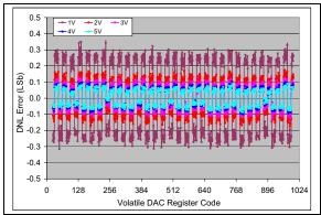
**FIGURE 2-77:** DNL vs. Code (code = 25 to 1000) and  $V_{REF}$  (MCP4716).  $V_{DD} = 5V$ ,  $V_{REF1}$ :  $V_{REF0} = '11'$ , G = '0',  $V_{REF} = 1V$ , 2V, 3V, 4V, and 5V,  $Temp = +25 ^{\circ}C$ .
