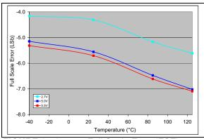
FIGURE 2-53: Full Scale Error (FSE) vs. Temperature (MCP4716).
