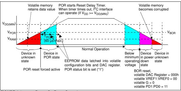
FIGURE 4-1: Power-On-Reset Operation.
