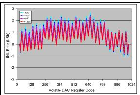
FIGURE 2-41: INL vs. Code (code = 25 to 1000) and Temperature (MCP4716).  $V_{DD} = 2.7V$ ,  $V_{REF1}$ :  $V_{REF0} = '11'$ , G = '0',  $V_{REF} = V_{DD}$ .
