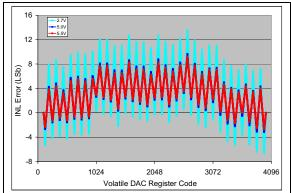
FIGURE 2-55: INL vs. Code (code = 100 to 4000) and  $V_{DD}$  (2.7V, 5V, 5.5V) (MCP4726).  $V_{REF1}$ :  $V_{REF0}$  = '10', G = '1',  $V_{REF}$  =  $V_{DD}$ /2,  $T_{CMD}$  = +25 °C.
