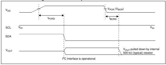
FIGURE 1-1: Power-On and Brown-Out Reset Waveforms.
