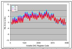
**FIGURE 2-19:** INL vs. Code (code = 100 to 4000) and Temperature (**MCP4726**).  $V_{DD} = 5V$ ,  $V_{REF1}$ :  $V_{REF0} = '10'$ , G = '0',  $V_{REF} = V_{DD}$ .
