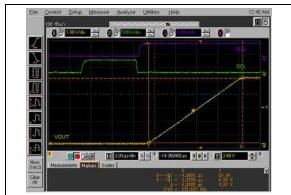
FIGURE 2-96: Full-Scale Settling Time (000h to FFFh) (MCP4726).
