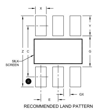
Units MILLIMETERS **Dimension Limits** MIN MOM MAX Contact Pitch Ε 0.95 BSC Contact Pad Spacing С 2.80 Contact Pad Width (X6) Χ 0.60 Contact Pad Length (X6) Υ 1.10 1.70 Distance Between Pads G Distance Between Pads GΧ 0.35 Overall Width 3.90
