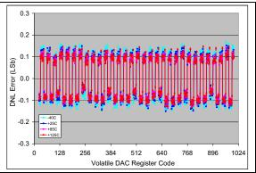
**FIGURE 2-47:** DNL vs. Code (code = 25 to 1000) and Temperature (MCP4716).  $V_{DD} = 2.7V$ ,  $V_{REF1}$ : $V_{REF0} = '11'$ , G = '0',  $V_{REF} = V_{DD}$ .
