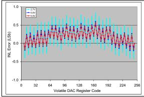
**FIGURE 2-57:** INL vs. Code (code = 6 to 250) and  $V_{DD}$  (2.7V, 5V, 5.5V) (MCP4706).  $V_{REF1}$ : $V_{REF0}$  = '10', G = '1',  $V_{REF}$  =  $V_{DD}$ /2,  $T_{CMD}$  = +25 °C.
