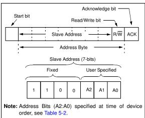
**FIGURE 5-9:** Slave Address Bits in the  $l^2C$  Control Byte.
