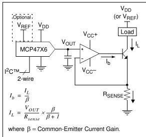
FIGURE 8-8: Digitally-Controlled Current Source.
