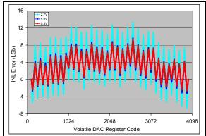
**FIGURE 2-61:** INL vs. Code (code = 100 to 4000) and  $V_{DD}$  (2.7V, 5V, 5.5V) (**MCP4726**).  $V_{REF1}$ : $V_{REF0}$  = '11', G = '1',  $V_{REF}$  =  $V_{DD}$ /2,  $T_{EMD}$  = +25 °C.
