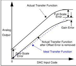
FIGURE 7-4: Gain Error and Full-Scale Error Example.
