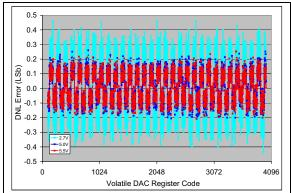
**FIGURE 2-64:** DNL vs. Code (code = 100 to 4000) and  $V_{DD}$  (2.7V, 5V, 5.5V) (**MCP4726**).  $V_{REF1}$ :  $V_{REF0}$  = '11', G = '1',  $V_{REF}$  =  $V_{DD}$ /2,  $T_{EMD}$  = +25 °C.
