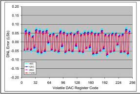
**FIGURE 2-45:** DNL vs. Code (code = 6 to 250) and Temperature (MCP4706).  $V_{DD} = 5V$ ,  $V_{REF1}$ : $V_{REF0} = '11'$ , G = '0',  $V_{REF} = V_{DD}$ .
