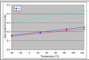
**FIGURE 2-50:** Zero Scale Error (ZSE) vs. Temperature (MCP4716).
