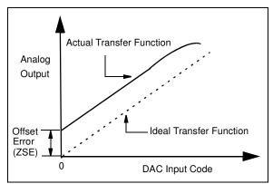
FIGURE 7-1: Offset Error Example.
