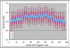
FIGURE 2-69: INL vs. Code (code = 6 to 250) and  $V_{REF}$  (MCP4706).  $V_{DD} = 5V$ ,  $V_{REF1}$ :  $V_{REF0} = '10'$ , G = '0',  $V_{REF} = 1V$ , 2V, 3V, 4V, and 5V,  $Temp = +25 ^{\circ}C$ .
