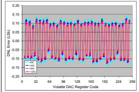
FIGURE 2-48: DNL vs. Code (code = 6 to 250) and Temperature (MCP4706).  $V_{DD} = 2.7V$ ,  $V_{REF1}$ :  $V_{REF0} = '11'$ , G = '0',  $V_{RFF} = V_{DD}$ .
