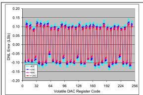
**FIGURE 2-30:** DNL vs. Code (code = 6 to 250) and Temperature (MCP4706).  $V_{DD} = 2.7V$ ,  $V_{REF1}$ : $V_{REF0} = '10'$ , G = '0',  $V_{REF} = V_{DD}$ .
