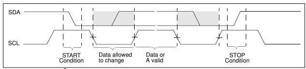
FIGURE 5-8: I<sup>2</sup>C Data States and Bit Sequence.
