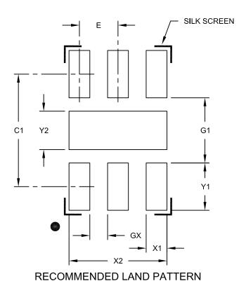
Units **MILLIMETERS** Dimension Limits MIN NOM MAX Contact Pitch 0.65 BSC Ε Optional Center Pad Width 1.00 Y2 Optional Center Pad Length Χ2 1.70 Contact Pad Spacing C1 2.10 Contact Pad Width (X6) X1 0.35 Contact Pad Length (X6) Y1 0.65 Distance Between Pads GX 0.20 Distance Between Pads G1 1.10
