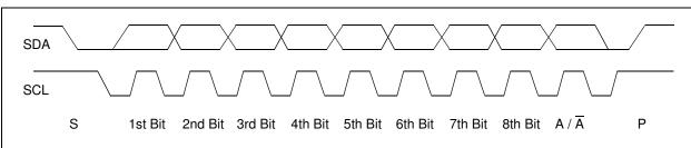
FIGURE 5-7: Typical 8-Bit I<sup>2</sup>C Waveform Format.
