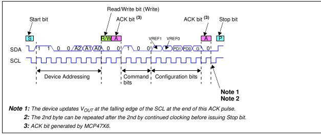
FIGURE 6-4: Write Volatile Configuration Bits Command.
