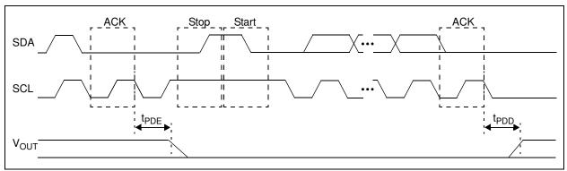
FIGURE 1-2: I<sup>2</sup>C Power-Down Command Timing.
