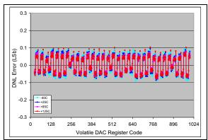
**FIGURE 2-26:** DNL vs. Code (code = 25 to 1000) and Temperature (MCP4716).  $V_{DD} = 5V$ ,  $V_{REF1}$ :  $V_{REF0} = '10'$ , G = '0',  $V_{REF} = V_{DD}$ .
