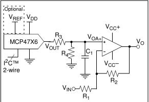
FIGURE 8-5: Digitally-Controlled Bipolar Voltage Source Example Circuit.
