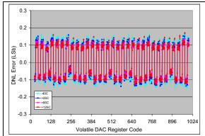
**FIGURE 2-11:** DNL vs. Code (code = 25 to 1000) and Temperature (MCP4716).  $V_{DD} = 2.7V$ ,  $V_{REF1}$ :  $V_{REF0} = '00'$ .
