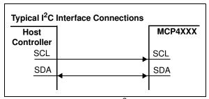
FIGURE 5-1: Typical I<sup>2</sup>C Interface.
