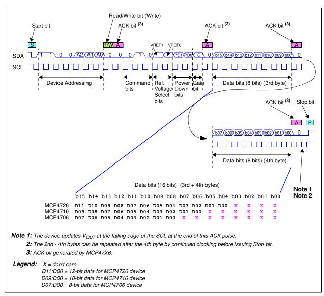
FIGURE 6-2: Write Volatile Memory Command.
