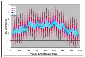
FIGURE 2-74: INL vs. Code (code = 25 to 1000) and  $V_{REF}$  (MCP4716).  $V_{DD} = 5V$ ,  $V_{REF1}$ : $V_{REF0} = '11'$ , G = '0',  $V_{RFF} = 1V$ , 2V, 3V, 4V, and 5V, Temp = +25 °C.
