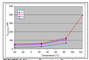
FIGURE 2-91: Powerdown Current vs. Temperature.  $V_{DD} = 2.7V$ , 3.3V, 4.5V, 5.0V and 5.5V, PD1:PD0 = '11'.
