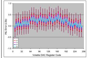
FIGURE 2-75: INL vs. Code (code = 6 to 250) and  $V_{REF}$  (MCP4706).  $V_{DD} = 5V$ ,  $V_{REF1}$ :  $V_{REF0} = '11'$ , G = '0',  $V_{REF} = 1V$ , 2V, 3V, 4V, and 5V,  $Temp = +25 ^{\circ}C$ .
