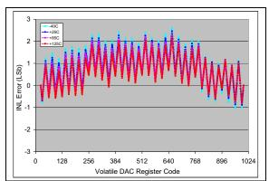
**FIGURE 2-5:** INL vs. Code (code = 25 to 1000) and Temperature (MCP4716).  $V_{DD} = 2.7V$ ,  $V_{REF1}$ :  $V_{REF0} = '00'$ .
