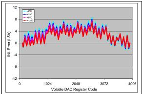
**FIGURE 2-37:** INL vs. Code (code = 100 to 4000) and Temperature (**MCP4726**).  $V_{DD} = 5V$ ,  $V_{REF1}$ :  $V_{REF0} = '11'$ , G = '0',  $V_{REF} = V_{DD}$ .
