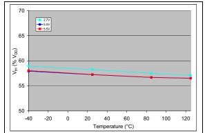
**FIGURE 2-92:**  $V_{IH}$  Threshold of SDA/SCL Inputs vs. Temperature and  $V_{DD}$ .
