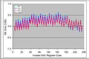
FIGURE 2-42: INL vs. Code (code = 6 to 250) and Temperature (MCP4706).  $V_{DD} = 2.7V$ ,  $V_{REF1}$ : $V_{REF0} = '11'$ , G = '0',  $V_{REF} = V_{DD}$ .
