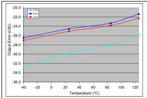
**FIGURE 2-85:** Output Error vs. Temperature (**MCP4726**).  $V_{DD} = 2.7V$  and 5V,  $V_{REF1}$ :  $V_{REF0} = '11'$ , G = '0',  $V_{REF} = V_{DD}$ , Code = 4000.
