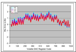
**FIGURE 2-2:** INL vs. Code (code = 25 to 1000) and Temperature (MCP4716).  $V_{DD} = 5V$ ,  $V_{REF1}$ : $V_{REF0} = '00'$ .
