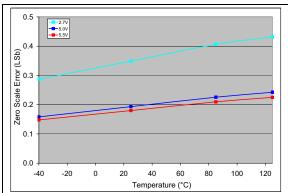
FIGURE 2-14: Zero Scale Error (ZSE) vs. Temperature (MCP4716).
