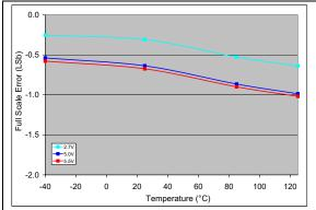
FIGURE 2-18: Full Scale Error (FSE) vs. Temperature (MCP4706).
