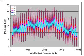
**FIGURE 2-67:** INL vs. Code (code = 100 to 4000) and  $V_{REF}$  (**MCP4726**).  $V_{DD} = 5V$ ,  $V_{REF1}$ :  $V_{REF0} = '10'$ , G = '0',  $V_{RFF} = 1V$ , 2V, 3V, 4V, and 5V,  $Temp = +25 \,^{\circ}$ C.
