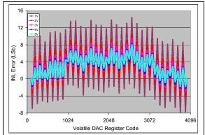
FIGURE 2-73: INL vs. Code (code = 100 to 4000) and  $V_{REF}$  (MCP4726).  $V_{DD} = 5V$ ,  $V_{REF1}$ :  $V_{REF0} = '11'$ , G = '0',  $V_{RFF} = 1V$ , 2V, 3V, 4V, and 5V,  $Temp = +25 \,^{\circ}$ C.
