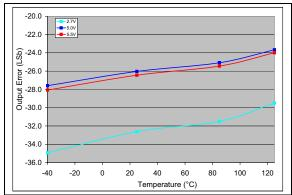
**FIGURE 2-79:** Output Error vs. Temperature (**MCP4726**).  $V_{DD} = 2.7V$  and 5V,  $V_{REF1}$ :  $V_{REF0} = '00'$ , Code = 4000.
