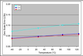
FIGURE 2-15: Zero Scale Error (ZSE) vs. Temperature (MCP4706).
