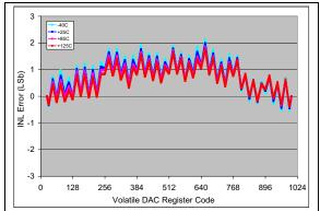
**FIGURE 2-38:** INL vs. Code (code = 25 to 1000) and Temperature (MCP4716).  $V_{DD} = 5V$ ,  $V_{REF1}$ :  $V_{REF0} = '11'$ , G = '0',  $V_{REF} = V_{DD}$ .
