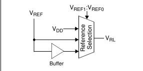
FIGURE 4-2: Resistor Ladder Reference Voltage Selection Block Diagram.
