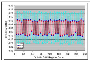
FIGURE 2-60: DNL vs. Code (code = 6 to 250) and  $V_{DD}$  (2.7V, 5V, 5.5V) (MCP4706).  $V_{REF1}$ :  $V_{REF0}$  = '10', G = '1',  $V_{REF}$  =  $V_{DD}$ /2,  $T_{CMD}$  = +25 °C.
