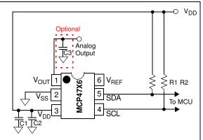
(a) Circuit when  $V_{DD}$  is selected as reference (Note:  $V_{DD}$  is connected to the reference circuit internally.)
