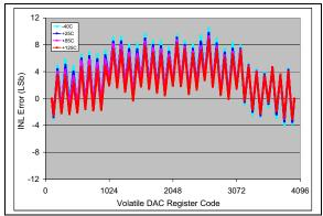
FIGURE 2-40: INL vs. Code (code = 100 to 4000) and Temperature (MCP4726).  $V_{DD} = 2.7V$ ,  $V_{REF1}$ :  $V_{REF0} = '11'$ , G = '0',  $V_{REF} = V_{DD}$ .
