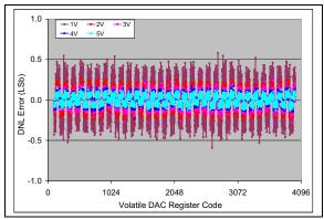
**FIGURE 2-76:** DNL vs. Code (code = 100 to 4000) and  $V_{REF}$  (**MCP4726**).  $V_{DD} = 5V$ ,  $V_{REF1}$ : $V_{REF0} = '11'$ , G = '0',  $V_{REF} = 1V$ , 2V, 3V, 4V, and 5V,  $T_{EMD} = +25$  °C.
