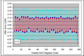
**FIGURE 2-66:** DNL vs. Code (code = 6 to 250) and  $V_{DD}$  (2.7V, 5V, 5.5V) (MCP4706).  $V_{REF1}$ : $V_{REF0}$  = '11', G = '1',  $V_{REF}$  =  $V_{DD}/2$ ,  $T_{EMD}$  = +25 °C.
