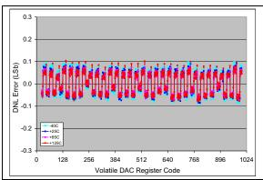
FIGURE 2-44: DNL vs. Code (code = 25 to 1000) and Temperature (MCP4716).  $V_{DD} = 5V$ ,  $V_{REF1}$ :  $V_{REF0} = '11'$ , G = '0',  $V_{REF} = V_{DD}$ .
