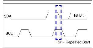
FIGURE 5-5: Repeat Start Condition Waveform.
