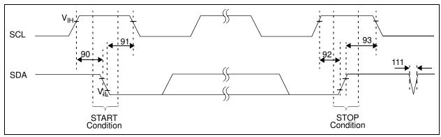
**FIGURE 1-3:** I<sup>2</sup>C Bus Start/Stop Bits Timing Waveforms.
