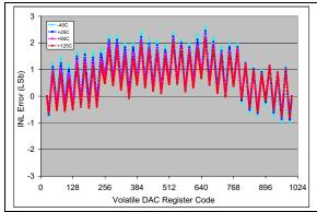
**FIGURE 2-23:** INL vs. Code (code = 25 to 1000) and Temperature (MCP4716).  $V_{DD} = 2.7V$ ,  $V_{REF1}$ :  $V_{REF0} = '10'$ , G = '0',  $V_{REF} = V_{DD}$ .
