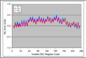
**FIGURE 2-21:** INL vs. Code (code = 6 to 250) and Temperature (MCP4706).  $V_{DD} = 5V$ ,  $V_{REF1}$ :  $V_{REF0} = '10'$ , G = '0',  $V_{REF} = V_{DD}$ .
