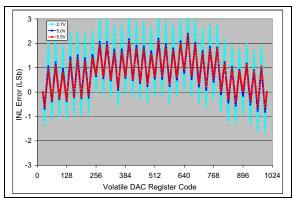
FIGURE 2-62: INL vs. Code (code = 25 to 1000) and  $V_{DD}$  (2.7V, 5V, 5.5V) (MCP4716).  $V_{REF1}$ : $V_{REF0}$  = '11', G = '1',  $V_{REF}$  =  $V_{DD}$ /2,  $V_{REF}$  = +25 °C.
