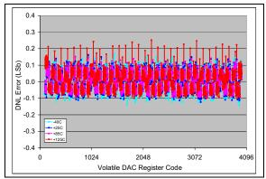
**FIGURE 2-25:** DNL vs. Code (code = 100 to 4000) and Temperature (**MCP4726**).  $V_{DD} = 5V$ ,  $V_{REF1}$ : $V_{REF0} = '10'$ , G = '0',  $V_{RFF} = V_{DD}$ .
