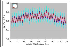
**FIGURE 2-63:** INL vs. Code (code = 6 to 250) and  $V_{DD}$  (2.7V, 5V, 5.5V) (MCP4706).  $V_{REF1}$ : $V_{REF0}$  = '11', G = '1',  $V_{REF}$  =  $V_{DD}$ /2,  $T_{CMD}$  = +25 °C.
