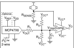
FIGURE 8-4: Single-Supply "Window" DAC.
