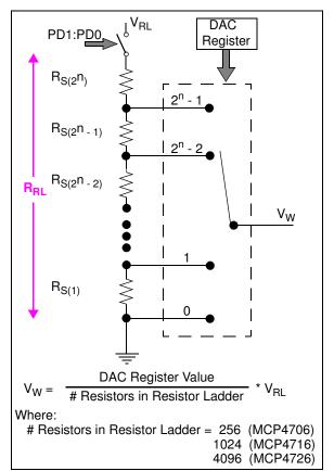
FIGURE 4-3: Resistor Ladder.
