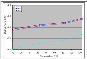
**FIGURE 2-80:** Output Error vs. Temperature (MCP4716).  $V_{DD} = 2.7V$  and 5V,  $V_{BFF1}$ :  $V_{BFF0} = '00'$ , Code = 1000.
