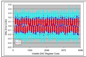
FIGURE 2-58: DNL vs. Code (code = 100 to 4000) and  $V_{DD}$  (2.7V, 5V, 5.5V) (**MCP4726**).  $V_{REF1}$ : $V_{REF0}$  = '10', G = '1',  $V_{REF}$  =  $V_{DD}$ /2,  $T_{CMD}$  = +25 °C.
