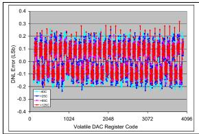
**FIGURE 2-46:** DNL vs. Code (code = 100 to 4000) and Temperature (**MCP4726**).  $V_{DD} = 2.7V$ ,  $V_{REF1}$ : $V_{REF0} = '11'$ , G = '0',  $V_{REF} = V_{DD}$ .
