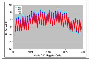
**FIGURE 2-22:** INL vs. Code (code = 100 to 4000) and Temperature (**MCP4726**).  $V_{DD} = 2.7V$ ,  $V_{REF1}$ : $V_{REF0} = '10'$ , G = '0',  $V_{RFF} = V_{DD}$ .
