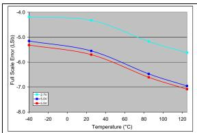
FIGURE 2-35: Full Scale Error (FSE) vs. Temperature (MCP4716).
