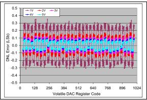
**FIGURE 2-71:** DNL vs. Code (code = 25 to 1000) and  $V_{REF}$  (MCP4716).  $V_{DD} = 5V$ ,  $V_{REF1}$ :  $V_{REF0} = '10'$ , G = '0',  $V_{REF} = 1V$ , 2V, 3V, 4V, and 5V,  $Temp = +25 \,^{\circ}C$ .
