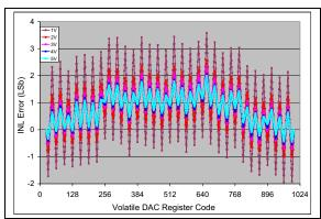
**FIGURE 2-68:** INL vs. Code (code = 25 to 1000) and  $V_{REF}$  (MCP4716).  $V_{DD} = 5V$ ,  $V_{REF1}$ : $V_{REF0} = '10'$ , G = '0',  $V_{REF} = 1V$ , 2V, 3V, 4V, and 5V, Temp = +25 °C.
