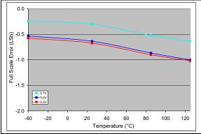
FIGURE 2-54: Full Scale Error (FSE) vs. Temperature (MCP4706).
