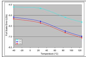
FIGURE 2-17: Full Scale Error (FSE) vs. Temperature (MCP4716).
