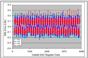
**FIGURE 2-10:** DNL vs. Code (code = 100 to 4000) and Temperature (**MCP4726**).  $V_{DD} = 2.7V$ ,  $V_{REF1}$ :  $V_{REF0} = '00'$ .
