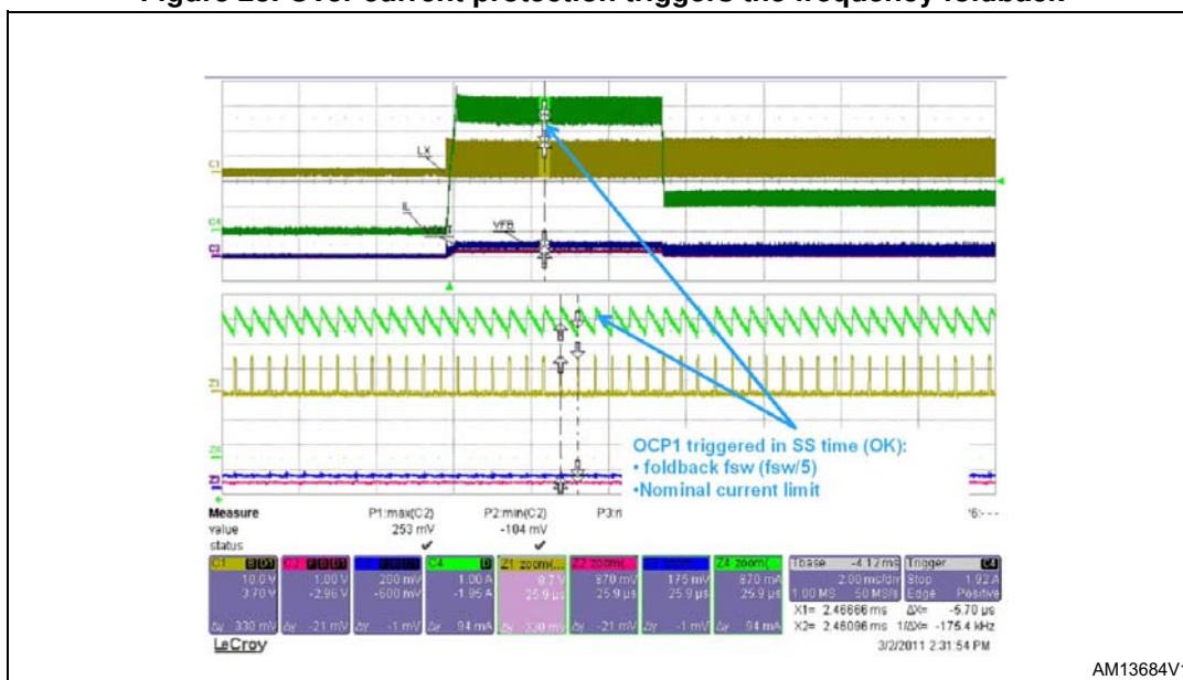
Figure 23. Over current protection triggers the frequency foldback
