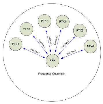
Figure 10. PRX using multiceiver
