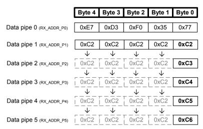
Figure 11. Addressing data pipes 0-5
