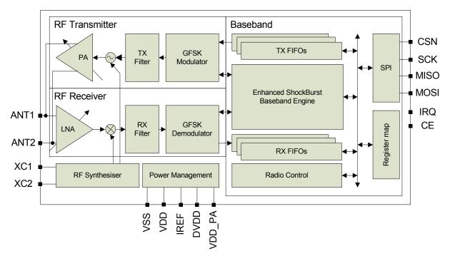
Figure 1. nRF24L01 block diagram
