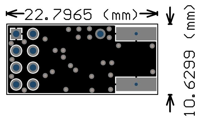
Figure 36. Bottom Layer (Module with OFM crystal and SMA connector)
