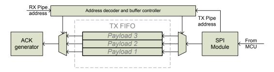
Figure 7. TX FIFO (PRX) with pending payloads
