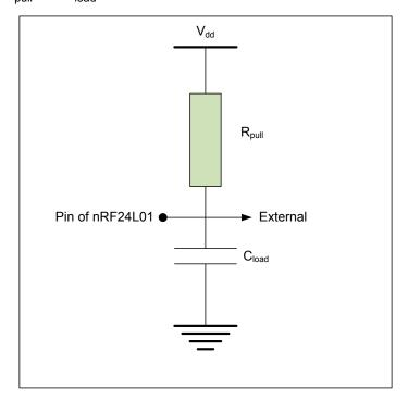
Figure 26. R<sub>pull</sub> and C<sub>load</sub>
