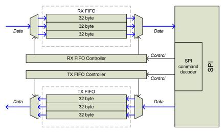
Figure 27. FIFO block diagram
