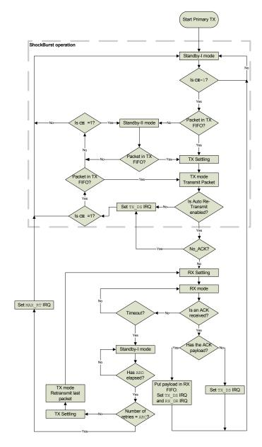
Figure 8. PTX operations in Enhanced ShockBurst™
