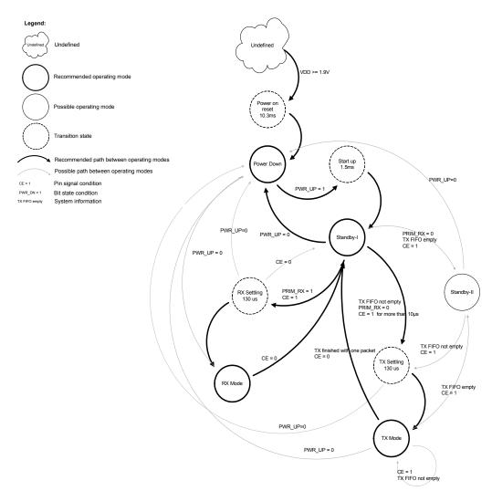
Figure 3. Radio control state diagram
