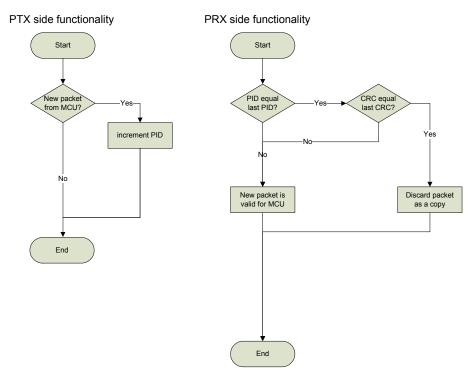
Figure 6. PID generation/detection
