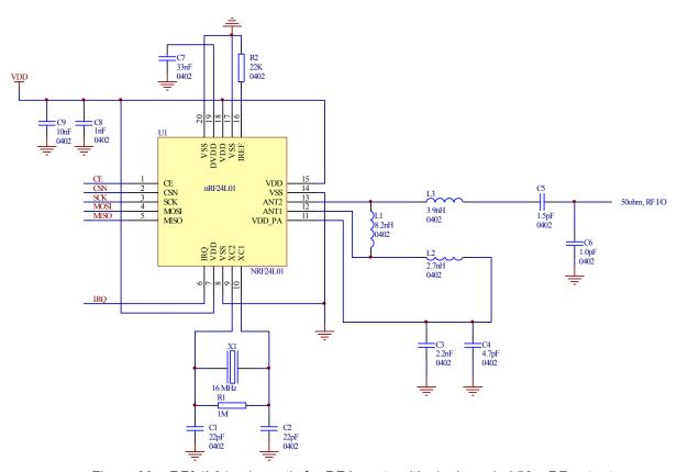
Figure 30. nRF24L01 schematic for RF layouts with single ended  $50\Omega$  RF output
