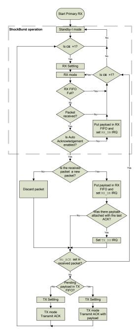
Figure 9. PRX operations in Enhanced ShockBurst™
