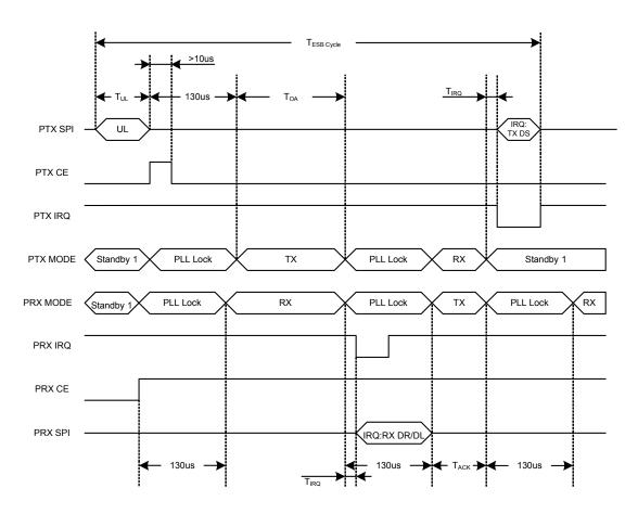
Figure 14. Timing of Enhanced ShockBurst™ for one packet upload (2Mbps)
