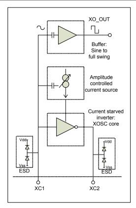
Figure 28. Principle of crystal oscillator
