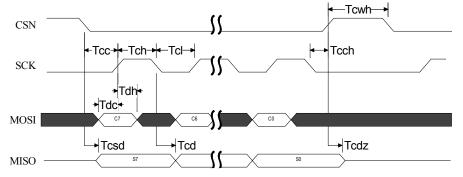
Figure 25. SPI NOP timing diagram
