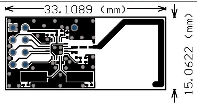
Figure 32. Top layer (nRF24L01 RF layout with single ended connection to PCB antenna and 0402 size passive components)
