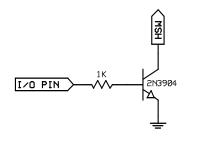
Switching circuit for the Propeller chip. Note: HIGH signal is required to turn on heater due to inversion of signal by the transistor.
