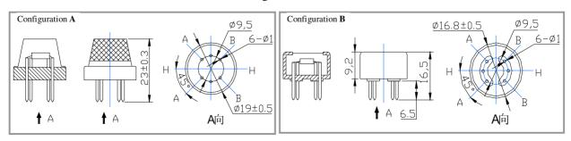
Structure and configuration of MQ-3 gas sensor is shown as Fig. 1 (Configuration A or B), sensor composed by micro AL<sub>2</sub>O<sub>3</sub> ceramic tube, Tin Dioxide (SnO<sub>2</sub>) sensitive layer, measuring electrode and heater are fixed into a crust made by plastic and stainless steel net. The heater provides necessary work conditions for work of sensitive components. The enveloped MQ-3 have 6 pin ,4 of them are used to fetch signals, and other 2 are used for providing heating current.
