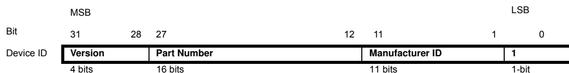
Figure 26-1. The Format of the Device Identification Register
