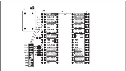
**Note:** Crystal circuits are very sensitive to noise and stray capacitances. In general, the traces between a crystal and a microcontroller should be as short as possible. The reason the PICDEM Mechatronics Demo Board strayed from good design practice was to give you the option to use pins RA7 and RA6 for other functions.
