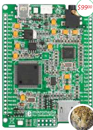
mikromedia for Stellaris M3 (features LM3S9B95)
