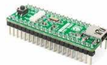
MIKROE-1367 MINI-M4 for STM32 contains STM32F415RG (ARM® Cortex™-M4)
