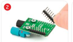
Turn the board upside down so that bottom side is facing you upwards. Place shorter pins of the header into the appropriate soldering pads.
