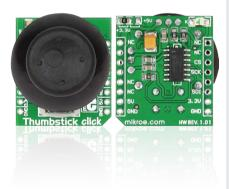
Thumbstick click<sup>™</sup> is a simple solution for adding an analog thumb joystick to your design. Along with the dual axis joystick unit, the board also carries an **MCP3204** 12-bit A/D converter. Thumbstick click<sup>™</sup> communicates with the target board microcontroller through **mikroBUS**<sup>™</sup> SPI (CS, SCK, MISO and MOSI) lines. The board is designed to use either a 3.3V or a 5V power supply.
