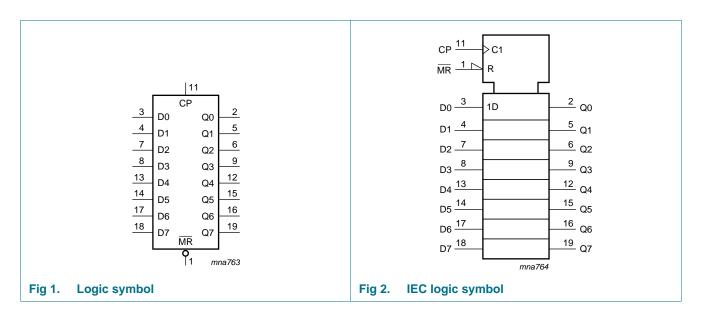
Octal D-type flip-flop with reset; positive-edge trigger
