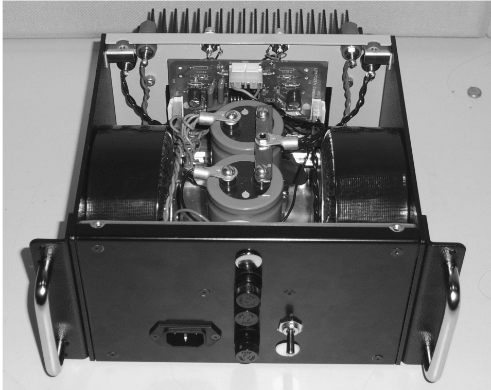
Figure 1. Complete LM4702-Based 100W/Channel High-Fidelity Power Amplifier
