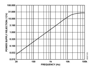
Figure 9. Power Supply Rejection vs. Frequency
