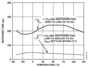
Figure 14.  $V_{\text{OUT}}$  Response Time for  $+V_{\text{S}}$  Power-Up/Power-Down vs. Temperature
