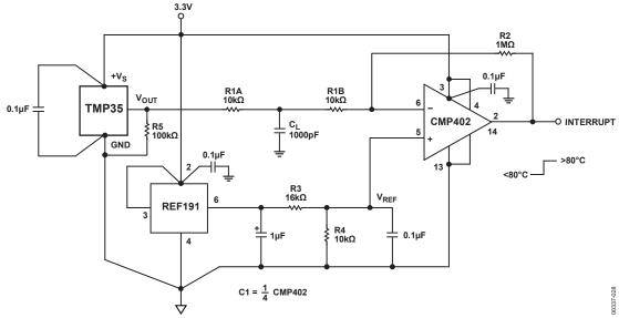
Figure 30. Microprocessor Overtemperature Interrupt Generator
