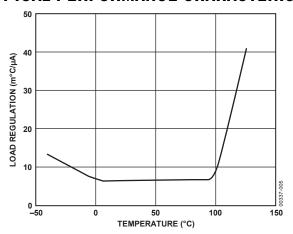
Figure 5. Load Regulation vs. Temperature ( $m^{\circ}C/\mu A$ )
