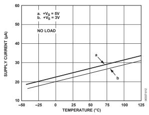
Figure 11. Supply Current vs. Temperature
