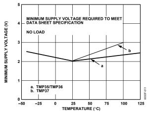
Figure 10. Minimum Supply Voltage vs. Temperature
