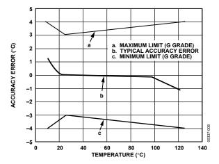
Figure 7. Accuracy Error vs. Temperature
