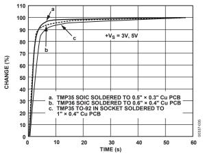
Figure 19. Thermal Response Time in Stirred Oil Bath
