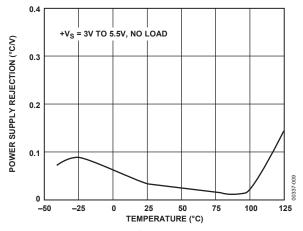
Figure 8. Power Supply Rejection vs. Temperature
