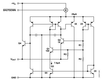
Figure 22. Temperature Sensor Simplified Equivalent Circuit
