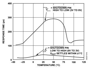
Figure 15.  $V_{OUT}$  Response Time for SHUTDOWN Pin vs. Temperature
