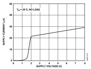
Figure 12. Supply Current vs. Supply Voltage
