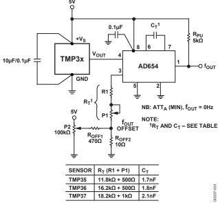
Figure 34. Temperature-to-Frequency Converter
