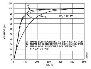
Figure 17. Thermal Response Time in Still Air
