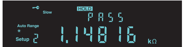
Limit compare mode on the DMM4020.
