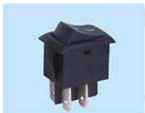
RSM2013 ON-OFF 10 A 125 VAC; 6 A 250 VAC DPST 4P
