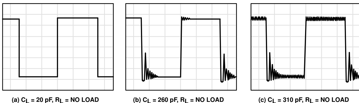
Figure 112. Effect of Capacitive Loads in Low-Bias Mode
