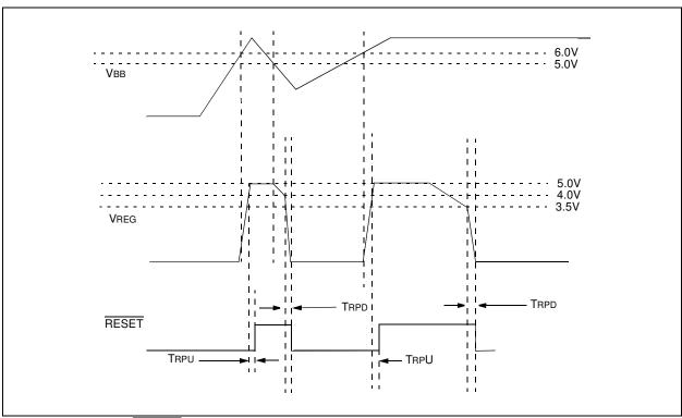
FIGURE 2-7: RESET Timing Diagram.
