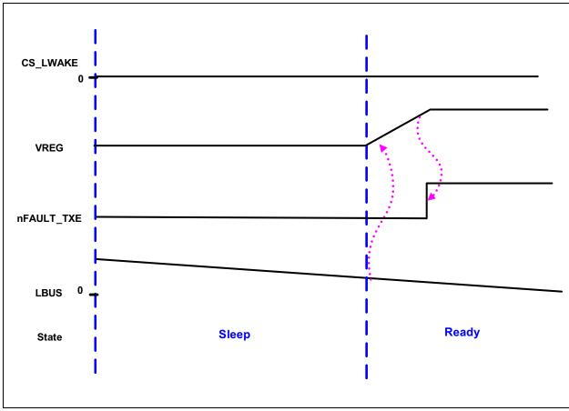
FIGURE 1-4: MCP2021P/2P Wake-Up Due to Bus Disconnecting.
