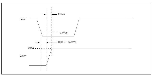
FIGURE 2-6: Regulator BUS WAKE Timing Diagram.
