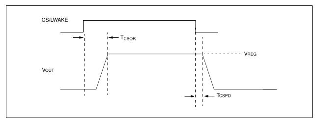
FIGURE 2-5: Regulator CS/LWAKE Timing Diagram.
