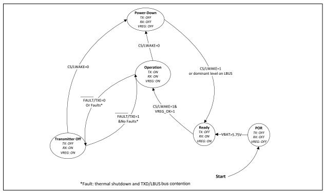
FIGURE 1-2: MCP2021/2 Operational Modes State Diagrams.
