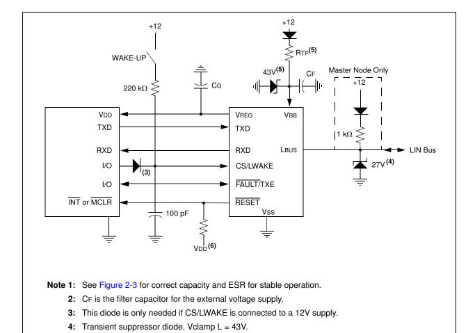
FIGURE 1-7: Typical MCP2022/MCP2022P Application.
