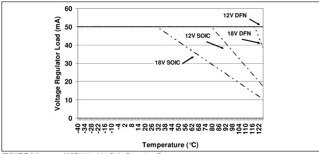
FIGURE 2-2: MCP2021-330 Safe Operating Range.
