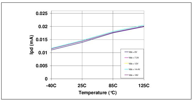
FIGURE 2-11: Typical I<sub>BBPD</sub> vs. Temperature.
