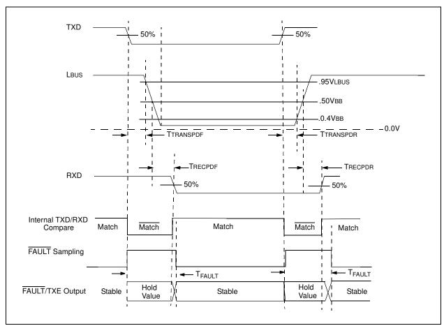
FIGURE 2-4: Bus Timing Diagram.
