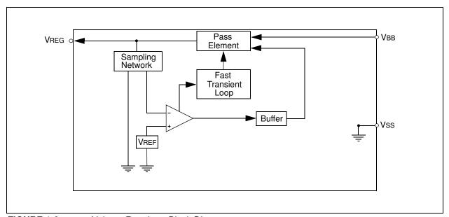
FIGURE 1-9: Voltage Regulator Block Diagram.
