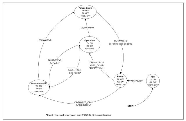
FIGURE 1-3: MCP2021P/2P Operational Modes State Diagrams.
