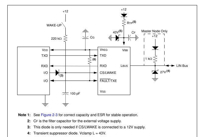
5: These components are required for additional load dump protection above 43V.
