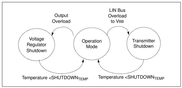
FIGURE 1-1: Thermal Shutdown State Diagrams.
