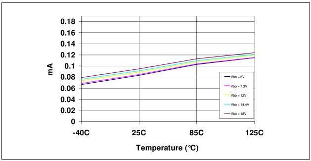
FIGURE 2-10: Typical I<sub>BBTO</sub> vs Temperature.
