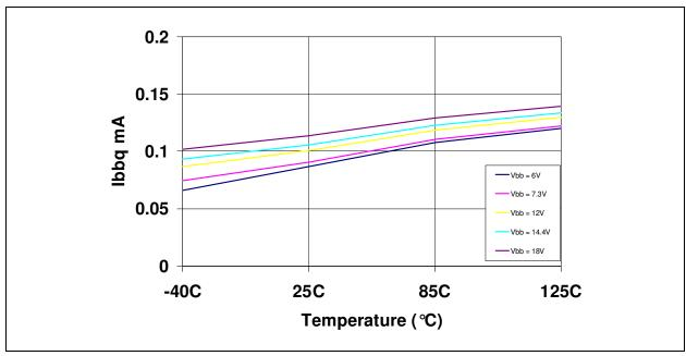
FIGURE 2-9: Typical I<sub>BBQ</sub> vs. Temperature.
