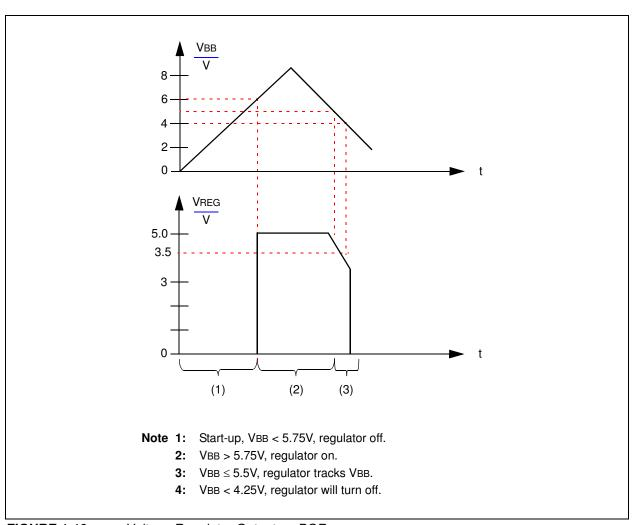
FIGURE 1-10: Voltage Regulator Output on POR.
