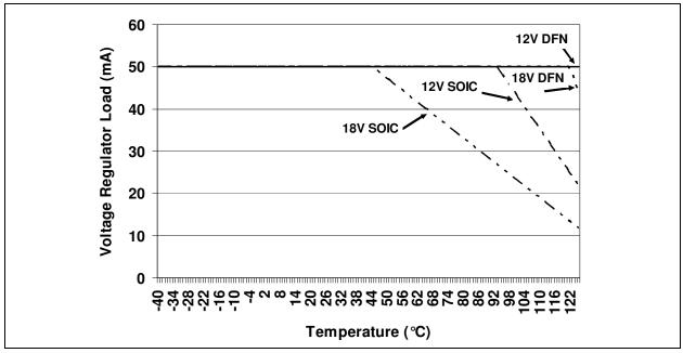
FIGURE 2-1: MCP2021-500 Safe Operating Range.
