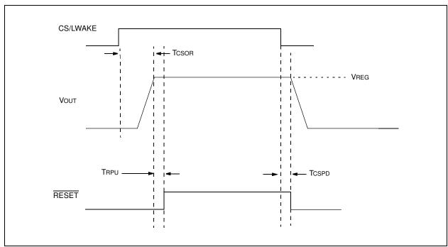
FIGURE 2-8: CS/LWAKE to RESET Timing Diagram.
