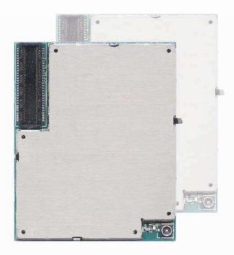
The SIM300 is a Tri-Band/Quad-Band\* GSM/GPRS solution in a compact plug-in module.
