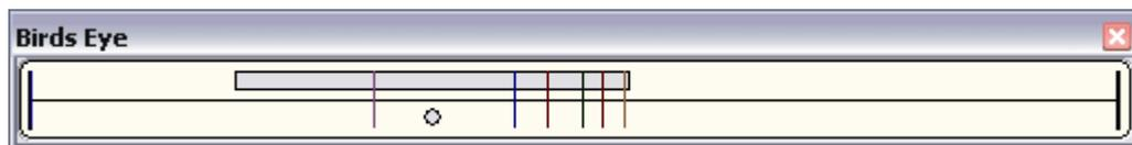
When the window is zoomed in on a small percentage of the data (usually the case) the waveform representation becomes a small circle so that you can still see it. Otherwise it would degenerate into a very thin line.
