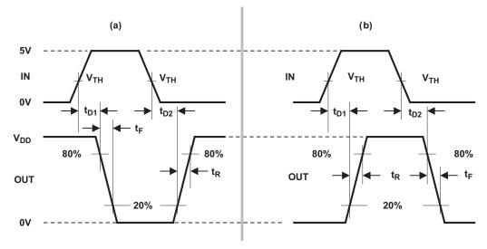
A. The 20% and 80% thresholds depict the dynamics of the BiPolar output devices that dominate the power MOSFET transition through the Miller regions of operation.
