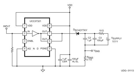
Figure 3. Sink Current Test Circuit
