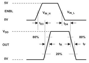
A. The 20% and 80% thresholds depict the dynamics of the BiPolar output devices that dominate the power MOSFET transition through the Miller regions of operation.
