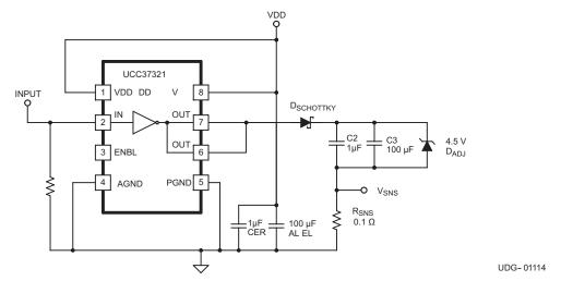
Figure 4. Source Current Test Circuit
