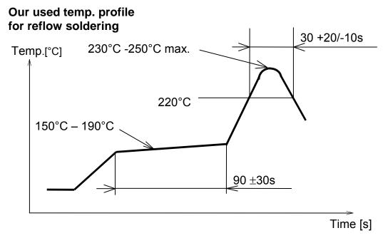
Reflow permissible cycle: 2 Opposite side reflow is prohibited due to module weight.
