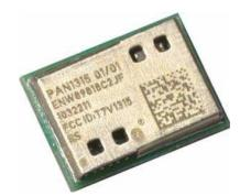
The above pictures show the laser marking on the top case, this is only an example from PAN1315.
