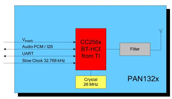
Note: The Slow Clock 32.768 kHz is mandatory, otherwise the module does not start up, refer to Chapter 5.4 for additional information.
