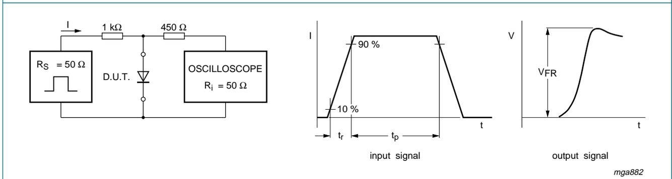
Input signal: forward pulse rise time  $t_r = 20 \text{ ns}$ ; forward current pulse duration  $t_p \geq 100 \text{ ns}$ ; duty cycle  $\delta \leq 0.005$
