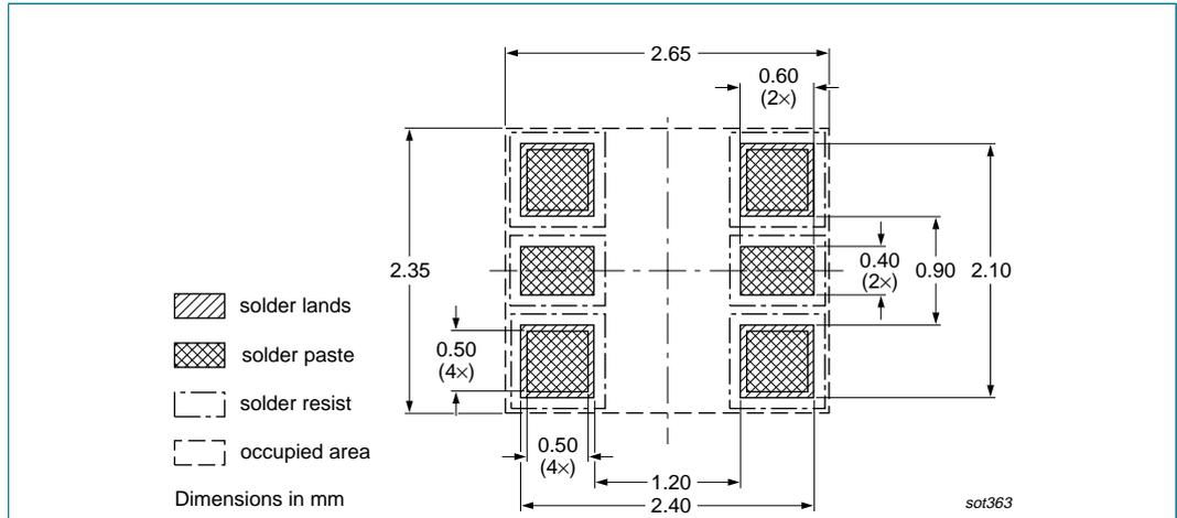
**Fig 15. Reflow soldering footprint BAV70S (SOT363/SC-88)**
