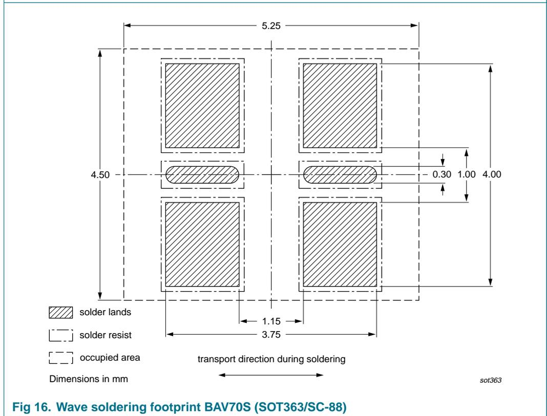
**Fig 16. Wave soldering footprint BAV70S (SOT363/SC-88)**
