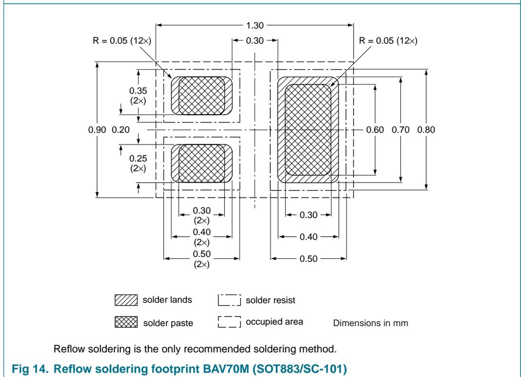
**Fig 14. Reflow soldering footprint BAV70M (SOT883/SC-101)**
