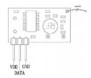
IF DATA pin is idle for more than 70mS, then the module will enter standby mode automatically.
