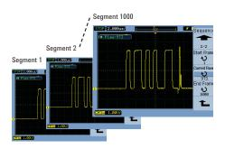
Figure 8. Use sequence mode to record up to 1000 triggers and review in playback mode for anomalies.
