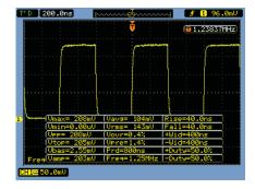
Figure 7. Display all single-channel measurements on screen simultaneously.
