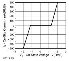
Fig. 5 - On-State Terminal Voltage vs. Terminal Current
