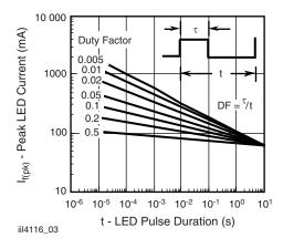
Fig. 3 - Peak LED Current vs. Duty Factor,  $\boldsymbol{\tau}$
