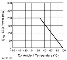
Fig. 6 - Maximum Output Power Dissipation
