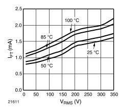
Fig. 7 - Trigger Current vs.
