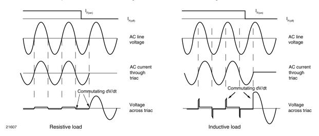
Fig. 8 - Waveforms of Resistive and Inductive Loads
