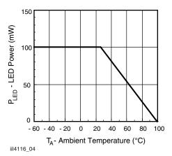
Fig. 4 - Maximum LED Power Dissipation
