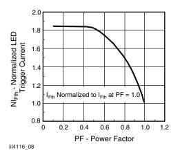
Fig. 10 - Normalized LED Trigger Current
