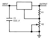
$V_{OUT} = 5V + (5V/R1 + I_Q) R2 5V/R1 > 3 I_Q,$ load regulation (L<sub>r</sub>)  $\approx$  [(R1 + R2)/R1] (L<sub>r</sub> of LM340-5).
