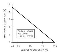
Figure 13. Maximum Power Dissipation vs T<sub>AMB</sub> for the TO-263 Package
