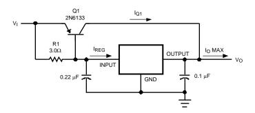
$$\begin{split} \beta(\text{Q1}) &\geq \frac{I_{O\,Max}}{I_{REG\,Max}} \\ \text{R1} &= \frac{0.9}{I_{REG}} = \frac{\beta(\text{Q1})\,V_{BE(\text{Q1})}}{I_{REG\,Max}(\beta\,+\,1)\,-\,I_{O\,Max}} \end{split}$$
