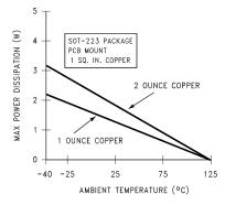
Figure 15. Maximum Power Dissipation vs T<sub>AMB</sub> for the SOT-223 Package
