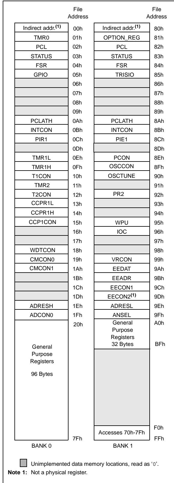
FIGURE 2-2: DATA MEMORY MAP OF THE PIC12F683
