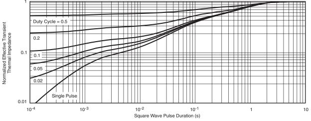
Normalized Thermal Transient Impedance, Junction-to-Foot
