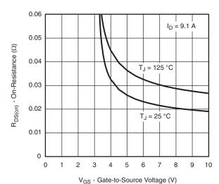
On-Resistance vs. Gate-to-Source Voltage
