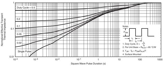
Normalized Thermal Transient Impedance, Junction-to-Ambient
