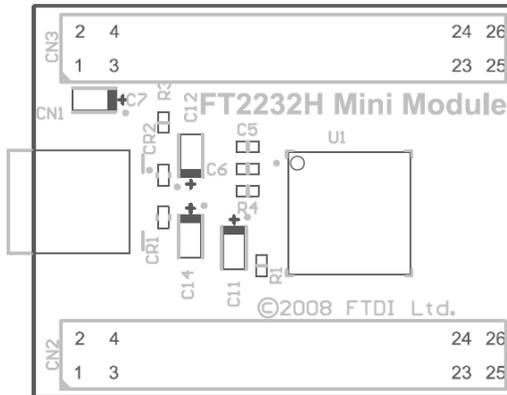
**Figure 3.1 FT2232H Mini Module Electrical Connections (Top View)**
