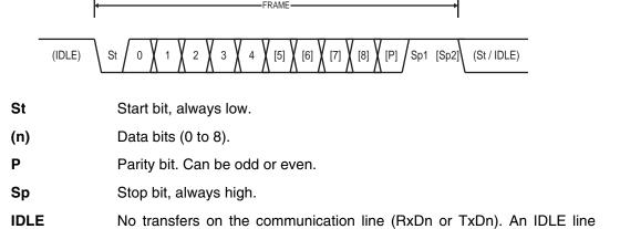
The frame format used by the USART is set by the UCSZn2:0, UPMn1:0 and USBSn bits in UCSRnB and UCSRnC. The Receiver and Transmitter use the same setting. Note that changing the setting of any of these bits will corrupt all ongoing communication for both the Receiver and Transmitter.
