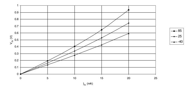
Figure 27-6. Output Low Voltage vs. Output Current, all I/Os excluding DP/DM, Vcc=5V
