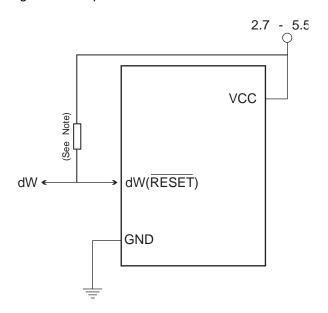
Figure 24-1 shows the schematic of a target MCU, with debugWIRE enabled, and the emulator connector. The system clock is not affected by debugWIRE and will always be the clock source selected by the CKSEL Fuses.
