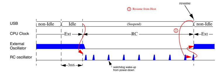
Figure 6-3. Example of clock switching with wake-up from Device
