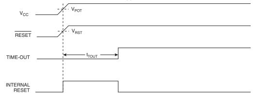
Figure 9-3. MCU Start-up, RESET Extended Externally
