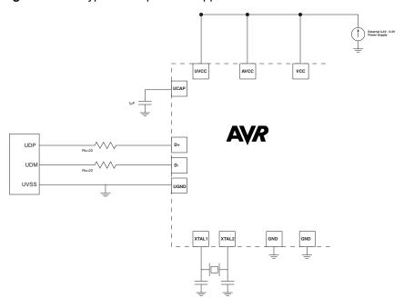
Figure 19-6. Typical Self powered application with 3.0V to 3.6 I/O
