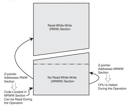
Figure 23-1. Read-While-Write vs. No Read-While-Write
