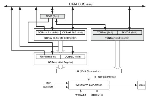
Figure 15-4. Output Compare Unit, Block Diagram
