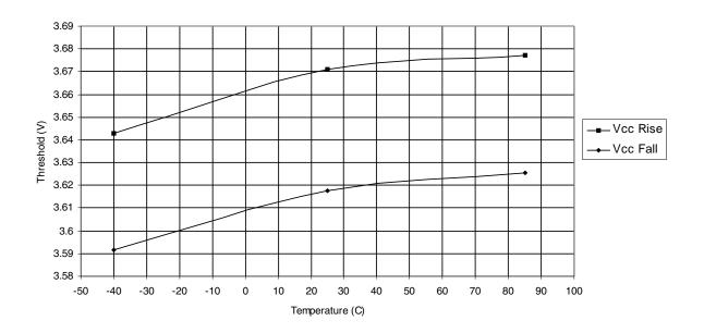
Figure 27-29. BOD Voltage (4.0V level) vs. Temperature
