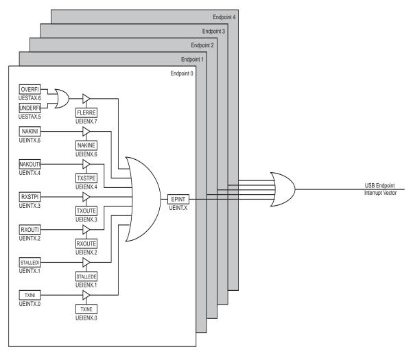
Figure 19-10. USB Endpoint Interrupt vector sources
