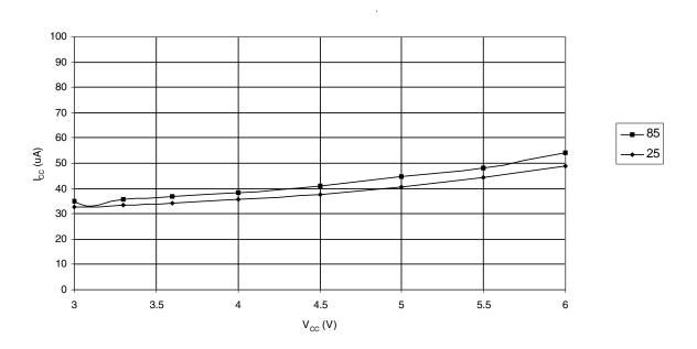
Figure 27-15. Power-down Supply Current vs. Vcc, with BOD Enabled, Regulator Enabled
