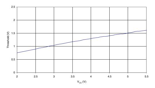
Figure 27-2. Input High Voltage vs. Vcc, all I/Os excluding DP/DM and MOSI/MISO
