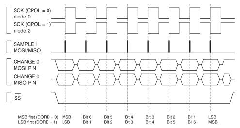
Figure 16-4. SPI Transfer Format with CPHA = 1
