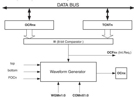
Figure 14-3. Output Compare Unit, Block Diagram
