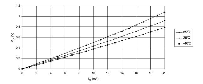
Figure 27-8. Output High Voltage vs. Output Current, all I/Os excluding DP/DM, Vcc=3V
