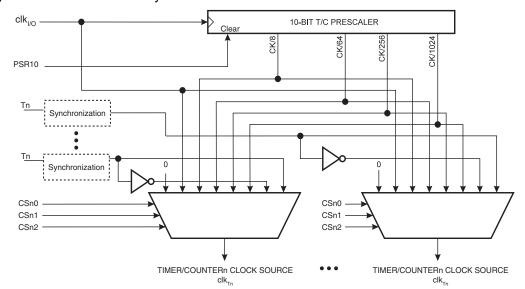
Figure 13-2. Prescaler for synchronous Timer/Counters
