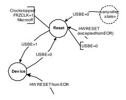
When the USB controller is in reset state:
