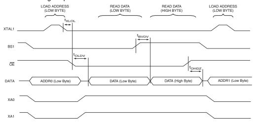
Note: 1. The timing requirements shown in Figure 25-7 (i.e., t<sub>DVXH</sub>, t<sub>XHXL</sub>, and t<sub>XLDX</sub>) also apply to reading operation.
