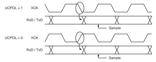
The UCPOLn bit UCRSC selects which XCKn clock edge is used for data sampling and which is used for data change. As Figure 17-3 shows, when UCPOLn is zero the data will be changed at rising XCKn edge and sampled at falling XCKn edge. If UCPOLn is set, the data will be changed at falling XCKn edge and sampled at rising XCKn edge.
