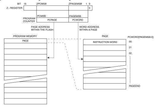
Figure 23-4. Addressing the Flash During SPM<sup>(1)</sup>
