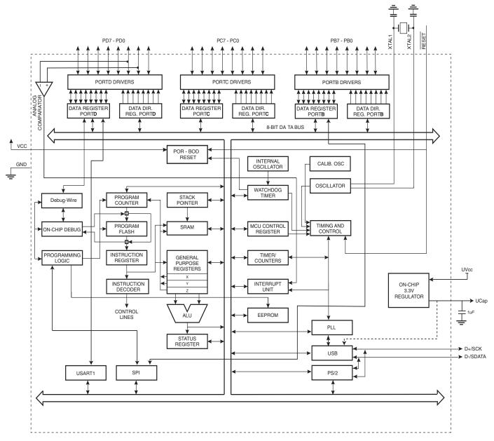
The AVR core combines a rich instruction set with 32 general purpose working registers. All the 32 registers are directly connected to the Arithmetic Logic Unit (ALU), allowing two independent registers to be accessed in one single instruction executed in one clock cycle. The resulting
