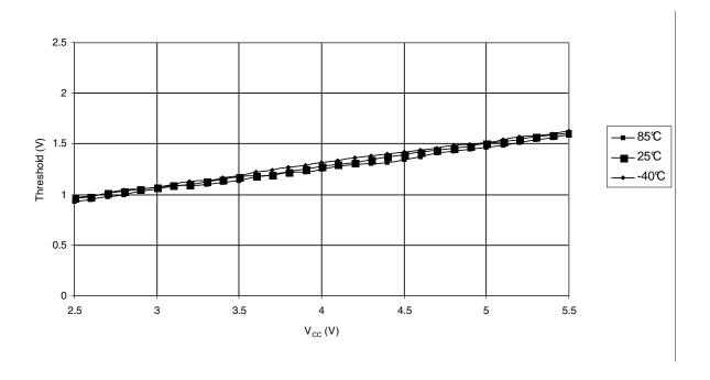
Figure 27-4. Input High Voltage vs. Vcc, MOSI/MISO I/Os
