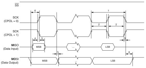
Table 26-3. SPI Interface Timing Requirements (Slave Mode)
