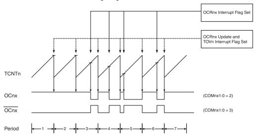
The Timer/Counter Overflow Flag (TOV0) is set each time the counter reaches TOP. If the interrupt is enabled, the interrupt handler routine can be used for updating the compare value.
