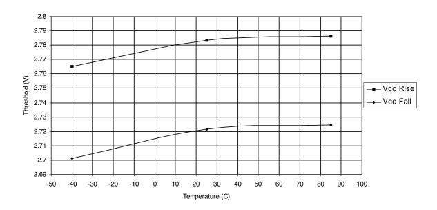
Figure 27-25. BOD Voltage (2.9V level) vs. Temperature
