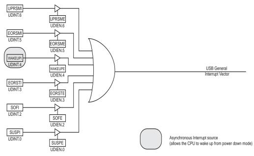
Each of these interupts are time-relative events that will be detected only if the USB clock is enabled (FRZCLK bit cleared), except for the WAKEUP interrupt that will trigger each time a state change is detected on the data lines.
