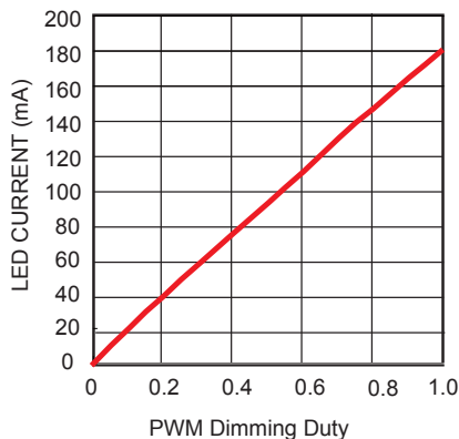
LED Current vs. PWM Dimming Duty
