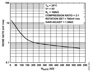
Figure 5. Noise Gate vs. R<sub>GATE</sub> (Pin 9 to V+)
