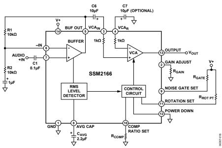
Figure 16. Functional Block Diagram and Typical Application
