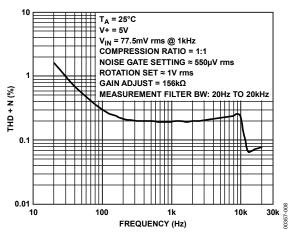
Figure 8. THD + N (%) vs. Frequency (Hz)
