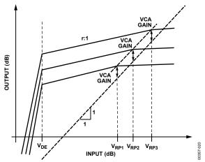
Figure 21. Effect of Varying the Rotation Point
