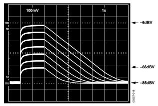
Figure 18. RMS Level Detector Performance with  $C_{AVG} = 22 \mu F$
