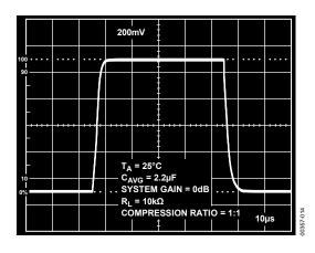
Figure 14. Large Signal Transient Response
