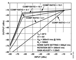
Figure 4. Output vs. Input Characteristics
