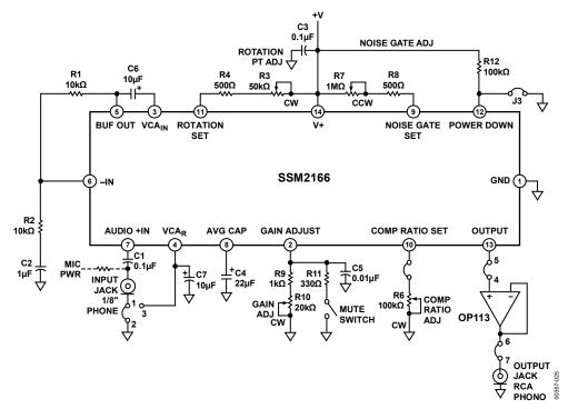
Figure 26. Evaluation Board Schematic
