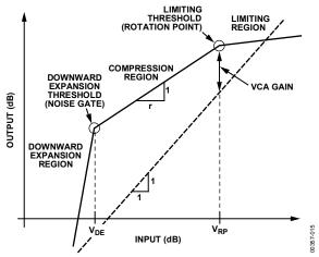
Figure 15. General Input/Output Characteristics
