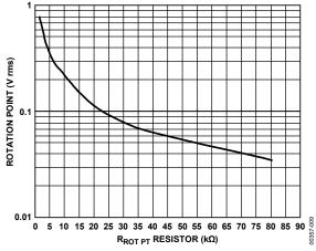
Figure 9. Rotation Point vs. R<sub>ROT PT</sub> (Pin 11 to V+)
