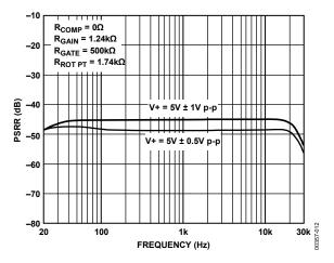
Figure 12. PSRR vs. Frequency
