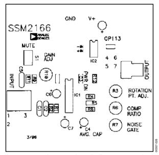
Figure 27. Evaluation Board Topside Silkscreen (Not to Scale)
