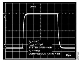
Figure 13. Small Signal Transient Response
