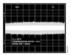
Figure 10. Wideband Peak-to-Peak Output Noise
