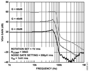
Figure 11. VCA Gain Bandwidth Curves vs. Frequency
