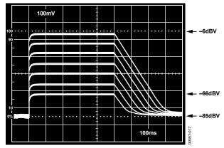
Figure 17. RMS Level Detector Performance with  $C_{AVG} = 2.2 \mu F$
