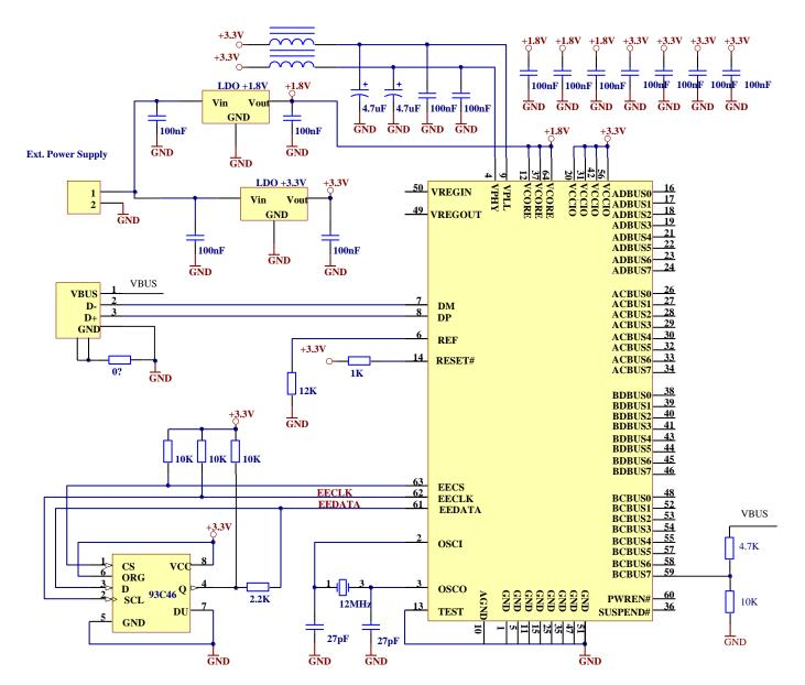
Figure 6.4 Self Powered Configuration Example 2
