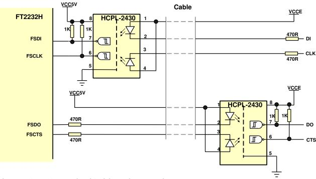
Figure 4.16 Fast Opto-Isolated Serial Interface Example
