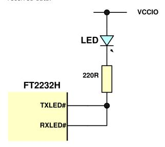
Figure 4.22 Single LED UART Configuration
