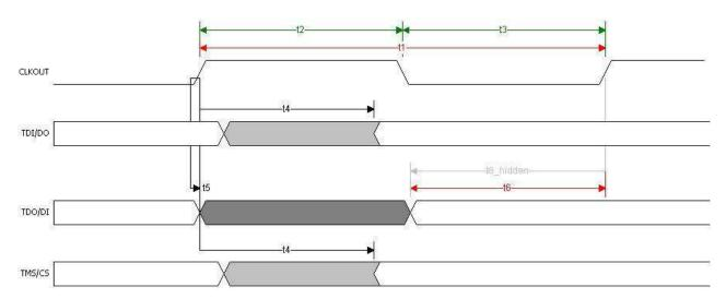
Figure 4.7 MPSSE Signal Waveforms
