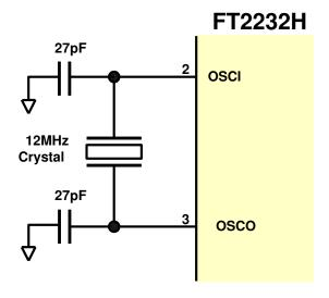
Figure 6.5 Recommended FT2232H Crystal Oscillator Configuration.
