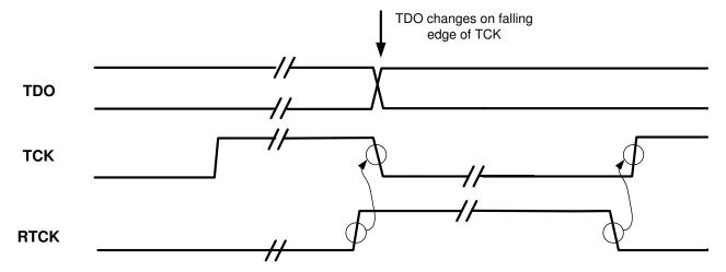
Figure 4.9: Adaptive Clocking waveform.
