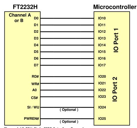
Figure 4.18 CPU-Style FIFO Interface Example
