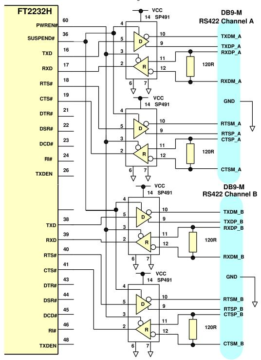
Figure 4.2 Dual RS422 Configuration
