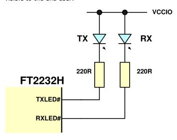
Figure 4.21 Dual LED UART Configuration
