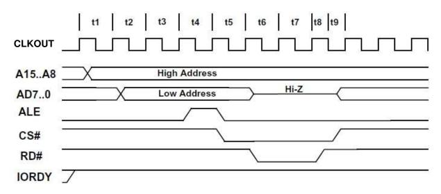
Figure 4.11 MCU Host Bus Emulation Mode Signal Waveforms - read cycle
