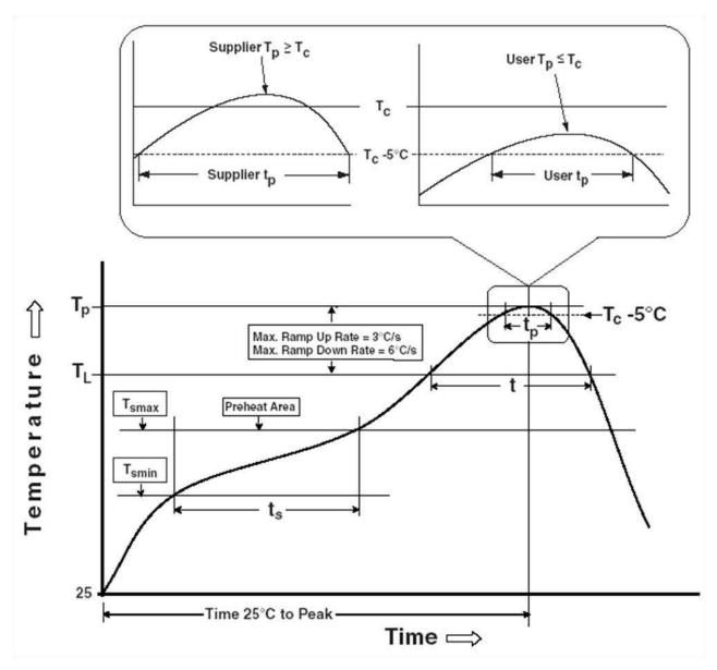
Figure 8.3 64 pin LQFP and QFN Reflow Solder Profile
