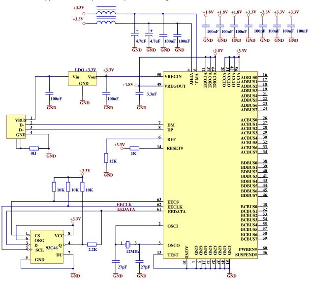
Figure 6.1 Bus Powered Configuration Example 1
