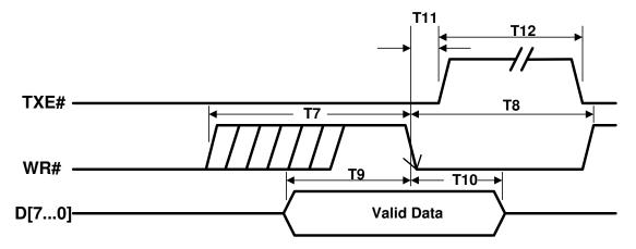
Figure 4.6 FT245 asynchronous FIFO Interface WRITE Signal Waveforms
