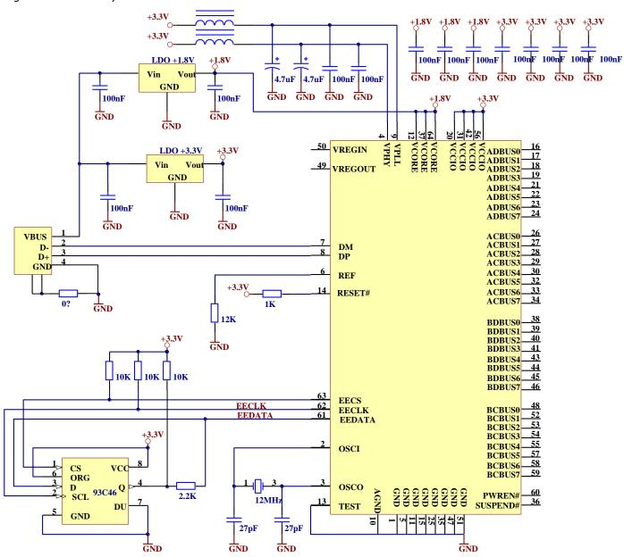
Figure 6.2 Bus Powered Configuration Example 2
