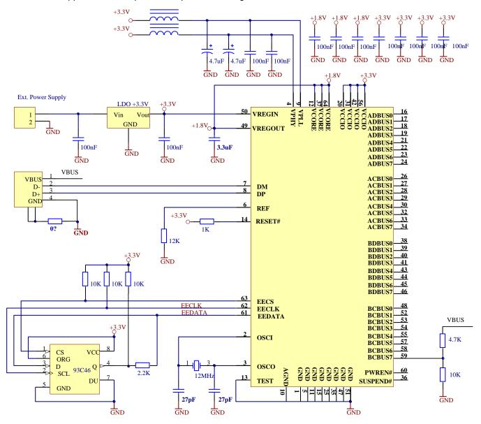
Figure 6.3 Self Powered Configuration Example 1
