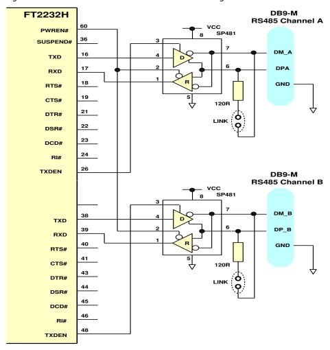
Figure 4.3 Dual RS485 Configuration
