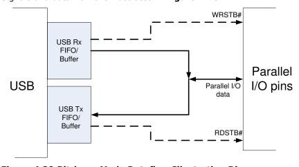
Figure 4.20 Bit-bang Mode Dataflow Illustration Diagram.
