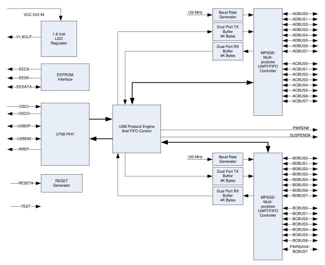
Figure 2.1 FT2232H Block Diagram
