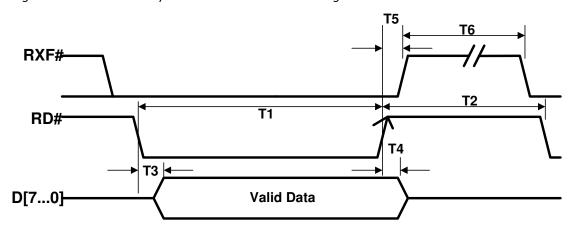
Figure 4.5 FT245 asynchronous FIFO Interface READ Signal Waveforms
