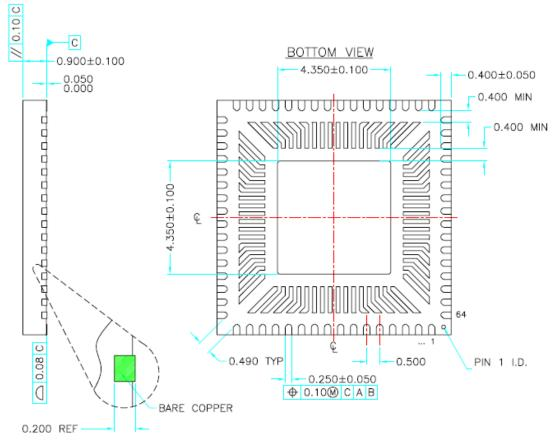
Figure 8.1 64 pin QFN Package Details
