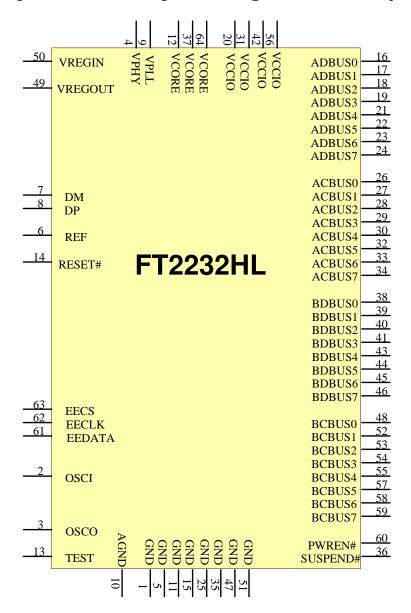
Figure 3.1 FT2232H Schematic Symbol
