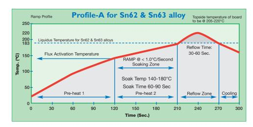
A profile utilizing a soak of up to two minutes at 155°C may help to minimize voiding in BGA assembles. This will allow more time for solvent components of the solder paste to outgas prior to reflow.
