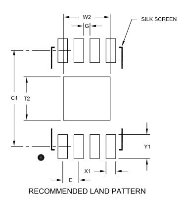
Units **MILLIMETERS Dimension Limits** MIN MAX MOM Contact Pitch Ε 0.50 BSC Optional Center Pad Width W2 1.46 1.36 Optional Center Pad Length T2 3.00 Contact Pad Spacing C1 Contact Pad Width (X8) X1 0.30 Contact Pad Length (X8) 0.75 Υ1 Distance Between Pads G 0.20
