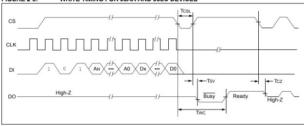
FIGURE 2-9: WRITE TIMING FOR 93C DEVICES
